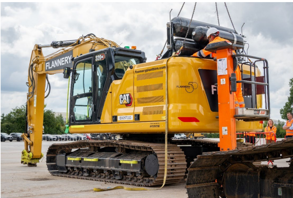
Figure 39 Tank installation on CAT320
