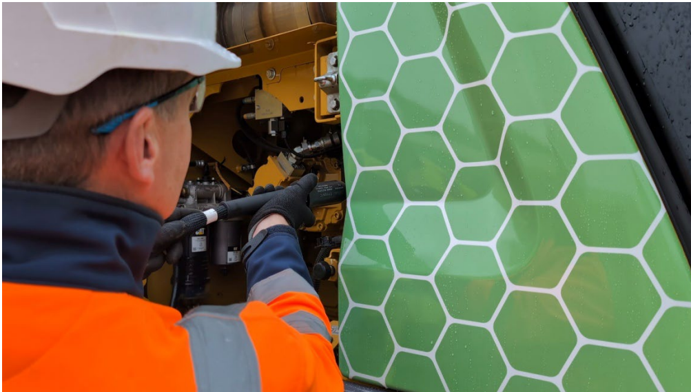
Figure 22 Excavator re-fuelling by the machine operator
