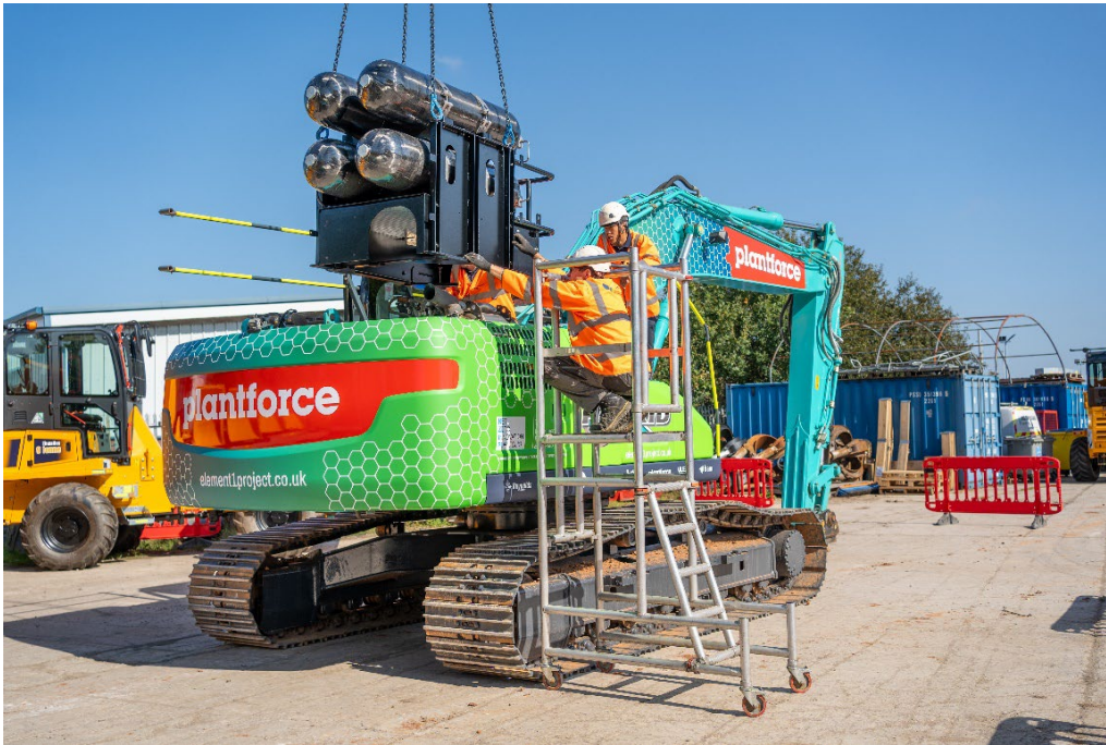
Figure 40 Tank installation on Kobelco SK210
