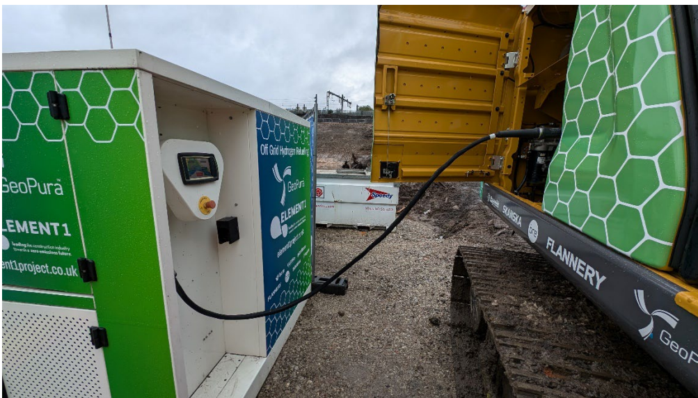
Figure 23 GeoPura HyQube dispenser hose connected to an excavator
