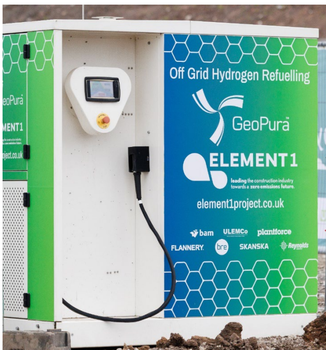
Figure 43 On site hydrogen dispenser
