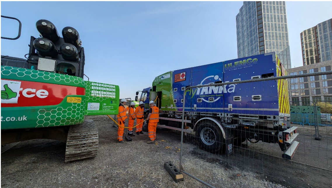
Figure 47 HyTanka® dispensing hydrogen on site in Manchester
