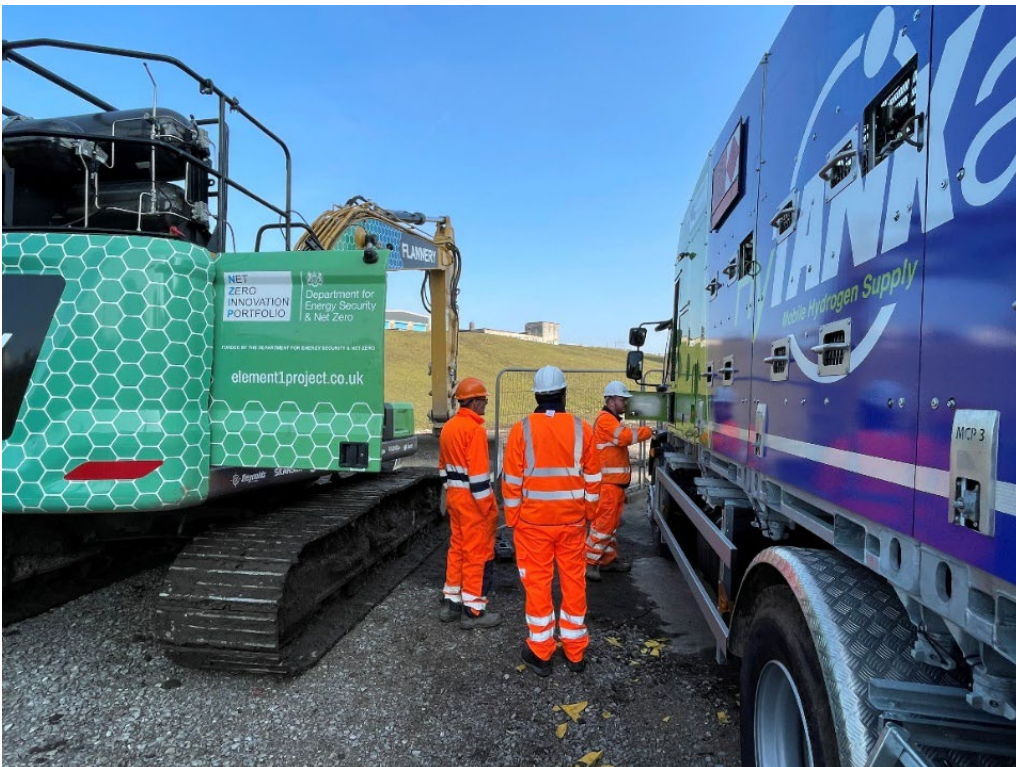
Figure 25 Refuelling the CAT machine with HyTANKa®
