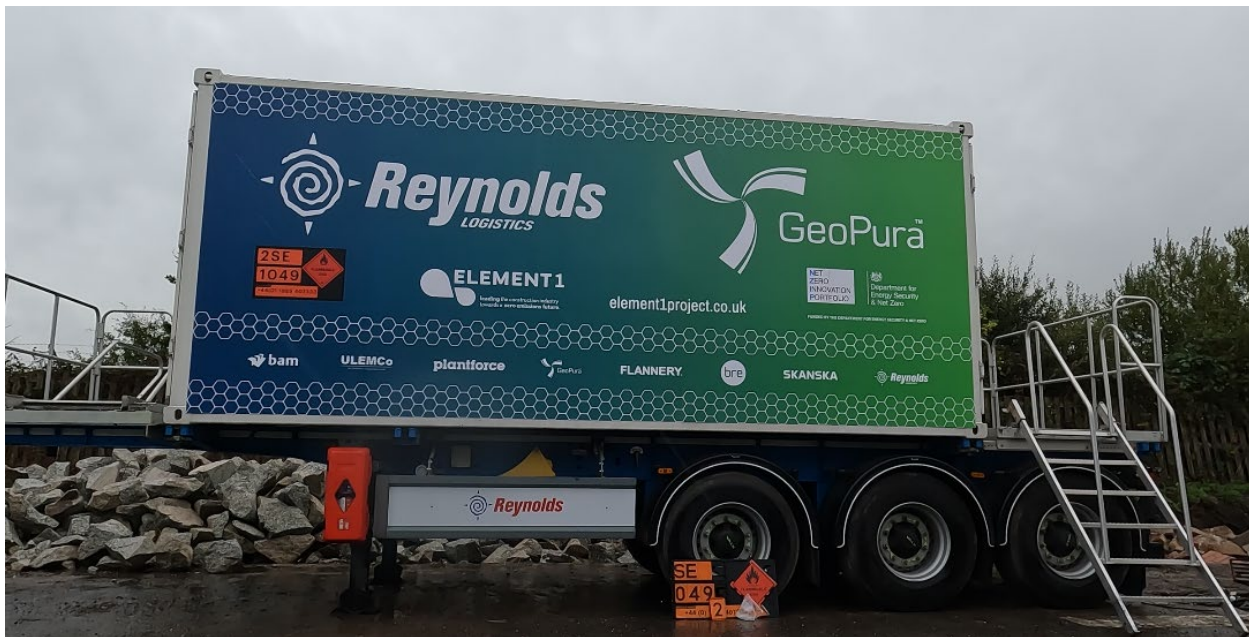
Figure 14 Multi Element Gas Container (MEGC)
