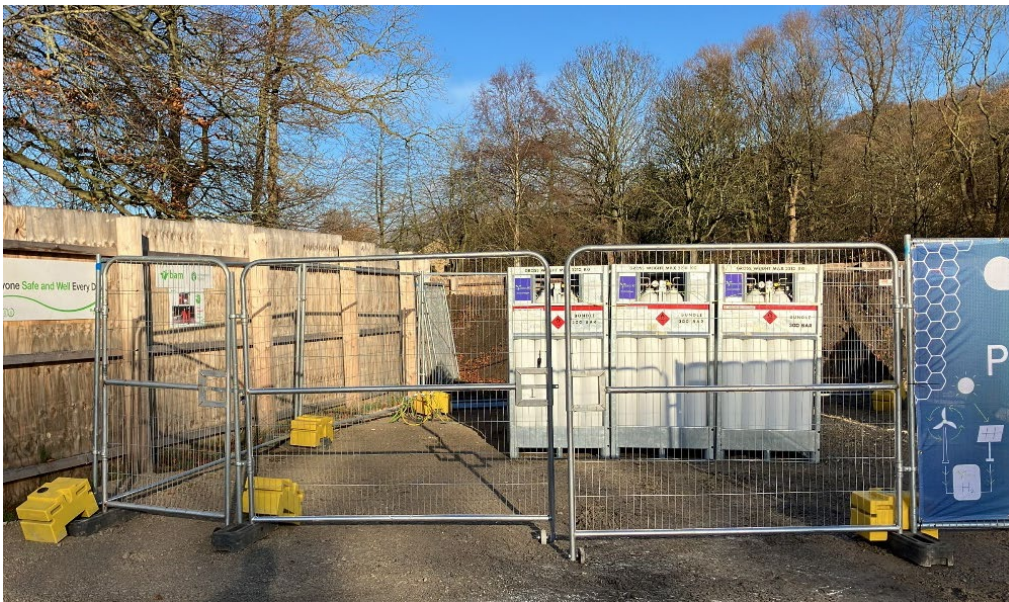
Figure 32 Hydrogen MCPs deployed at Brighthouse mitigating bowser delay
