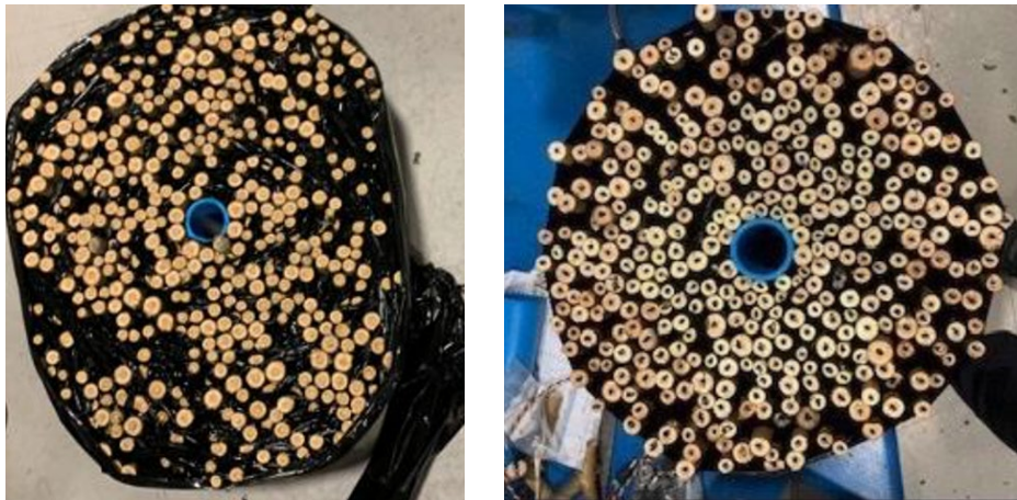
Figure 6: Iterated improvement of the bale mechanism illustrating greater uniformity.
