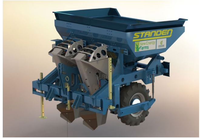
Figure 56: Initial CAD design work and the final CAD designs for the CEEDS™ planter. This is a 2-row fully automatic planter.
