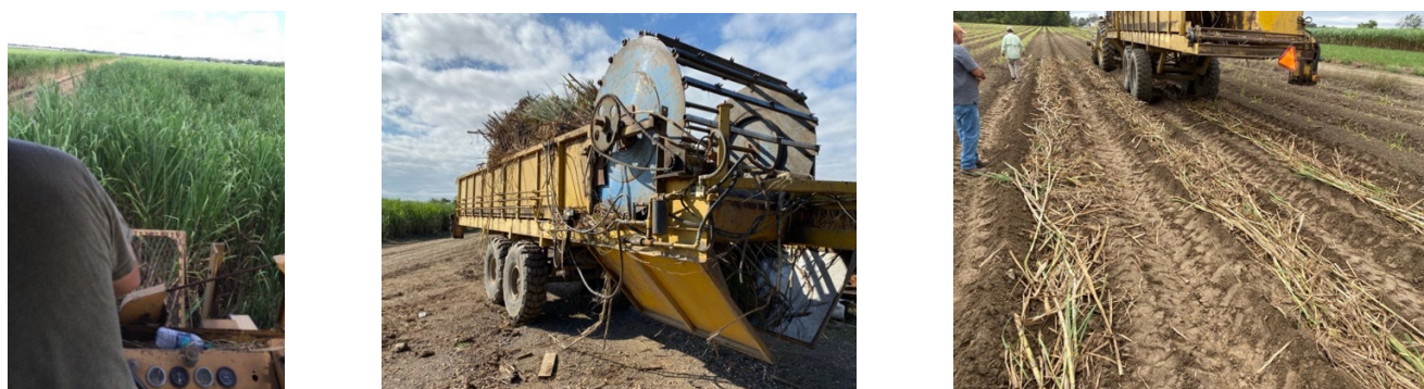
Figure 40: Left: Image of automated whole-stem sugarcane planting in whole-stem; Middle: Planter to lay in rows; Right: Final stem material in the rows before being covered up.
