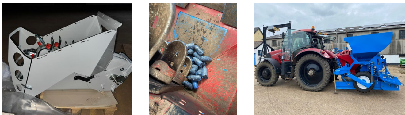
Figure 55: Images of testing CEEDS™ movement and pick up inside existing potato cup planter units, as well as the existing potato planter used for these trials.
