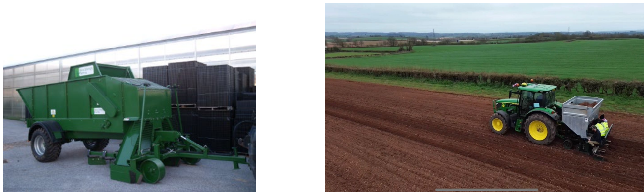
Figure 41: Miscanthus rhizome planting operations. Left: Automatic rhizome planter, WH Loxton Ltd; Right: Manual planter (Miscanthus Nurseries Ltd).
