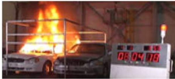
Figure 9. Photograph of the experiment involving two cars at around 500 s, taken from Park et al. [15]
