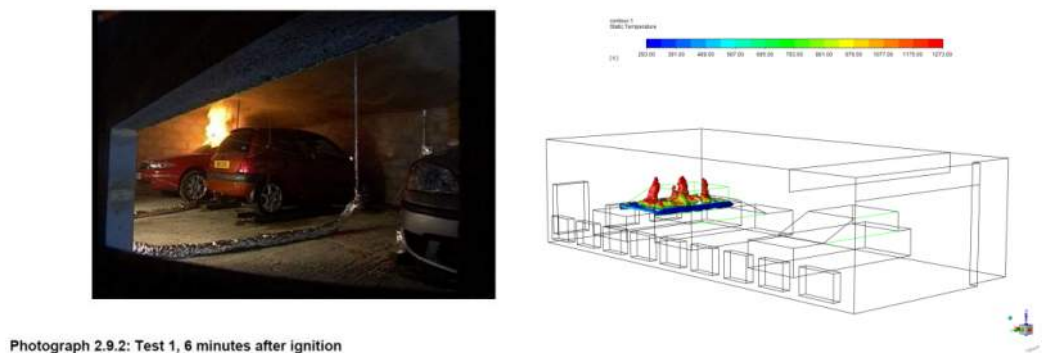
Fig. 5. Flame shape at 180 s of the analysis (6 th minute of the experiment)
