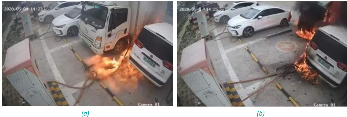
Figure 24. Fire in an open-air car park (a) ignition of neighbouring vehicle's tyre at around 40 s after the initiation of thermal runaway of the battery in the charging EV, (b) ignition of the rear of the third vehicle in the row
