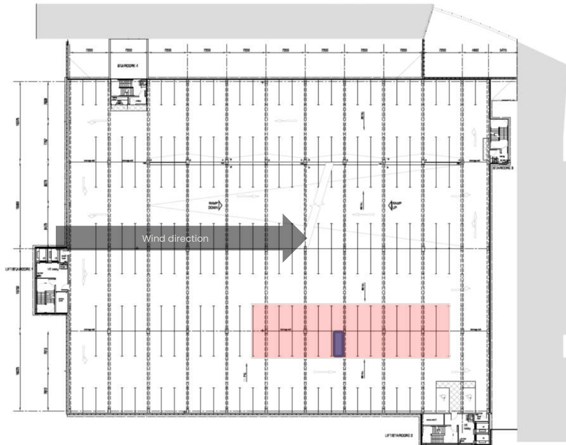
Figure 20. Level 3 car park layout showing location of the initiating vehicle and estimated area of fire spread over 30 vehicles
