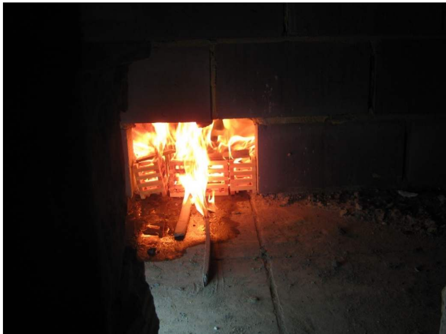
Figure 27 – Ignition source within hearth of cladding rig
