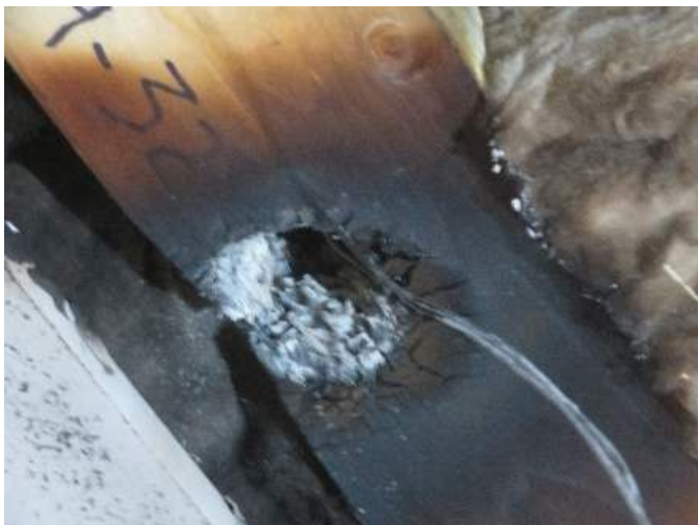
Figure 97 – Localised charring/smouldering at location of thermocouple installation
