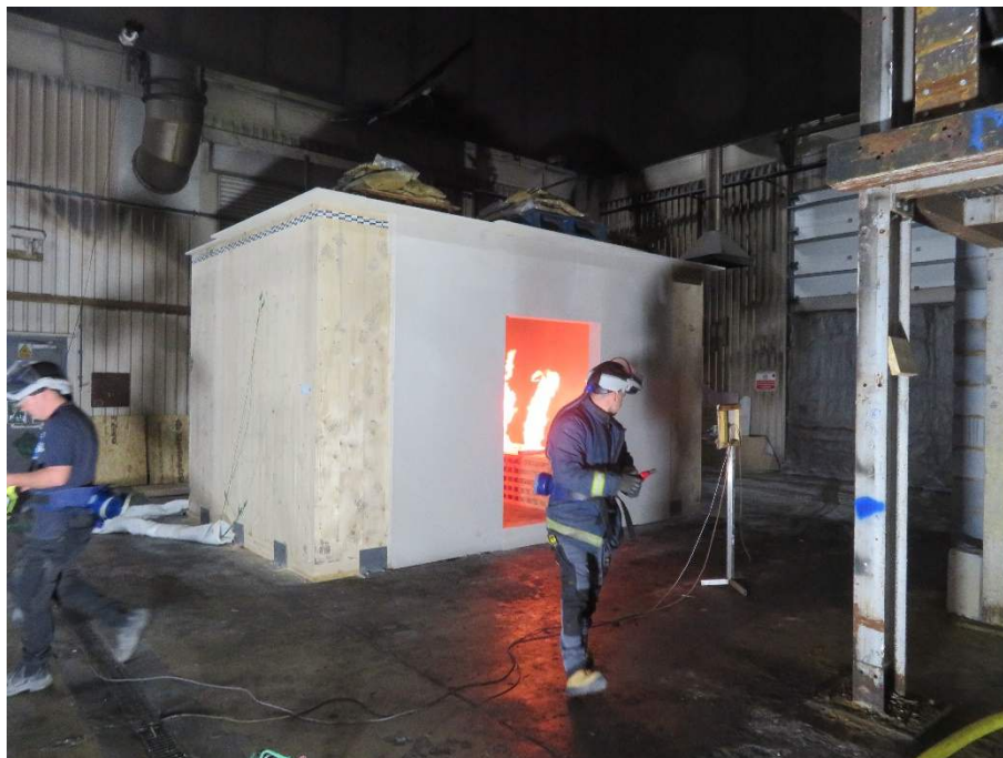
Figure 59 – Ignition of the fire load in the CLT-protected compartment
