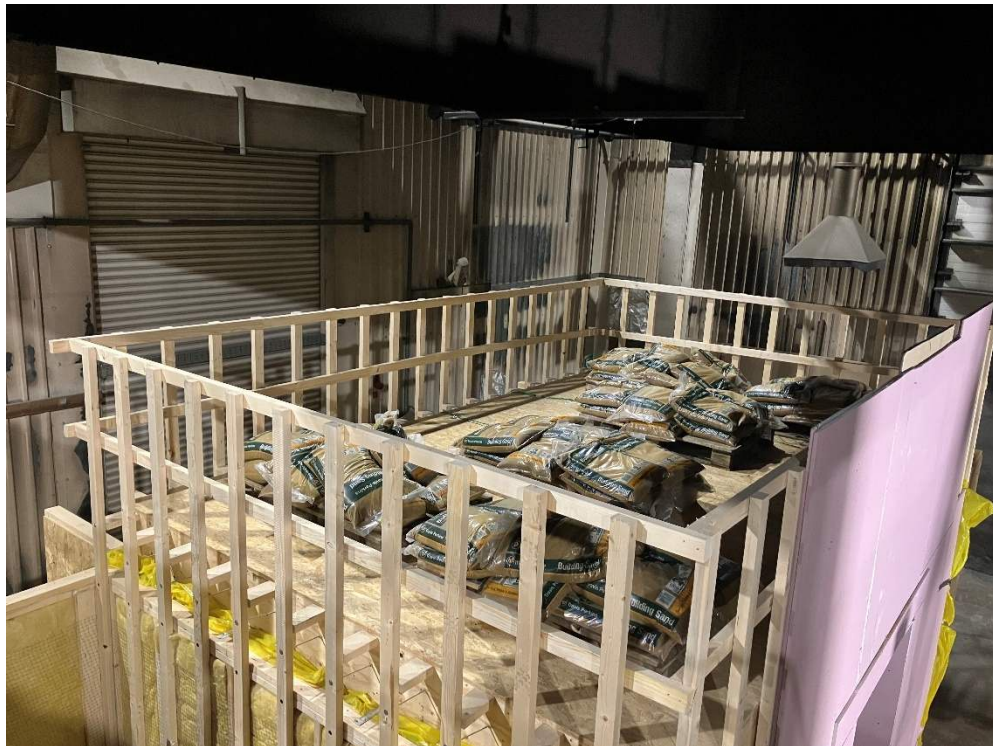
Figure 79 – View from above showing protection to opening and floor load
