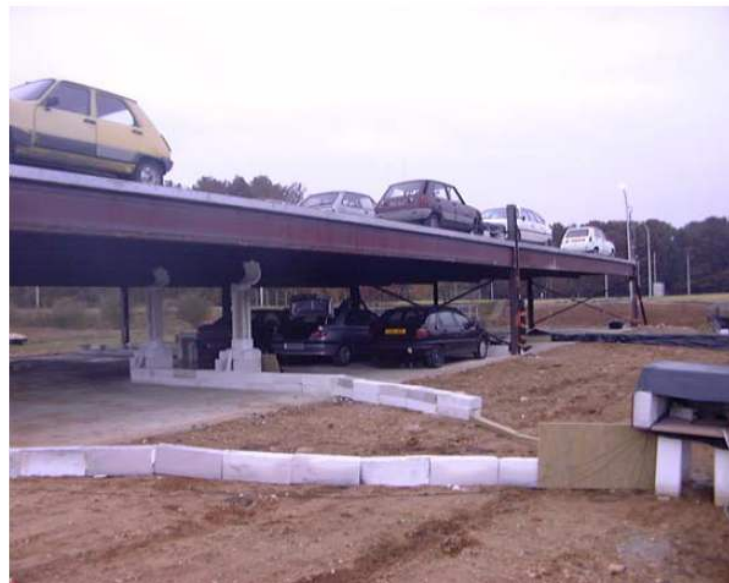
Figure 6 – The open car park configuration used in the tests sponsored by ECSC 14 . This is for the setup in test 2.
