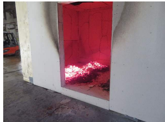
Burn out of the movable fire load (60 minutes)
