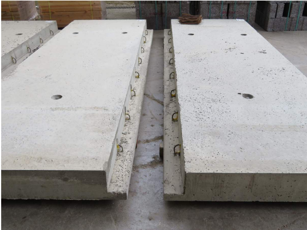
Figure 1 – Precast planks used to form the roof of the fire compartment
