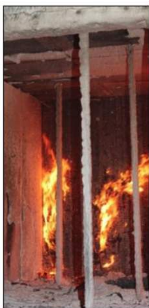
Premature delamination of the CLT
