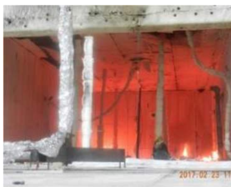
Test 1-2 – gypsum boards remained: 1 layer on the ceiling and 2 layers on the walls
