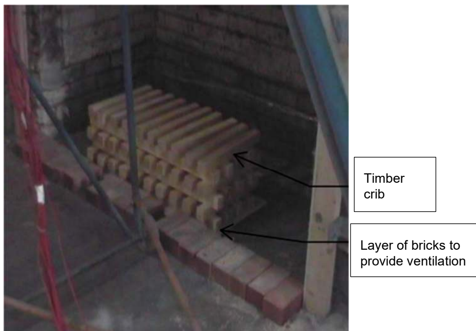
Figure 16 – Crib located within the hearth of the cladding rig
