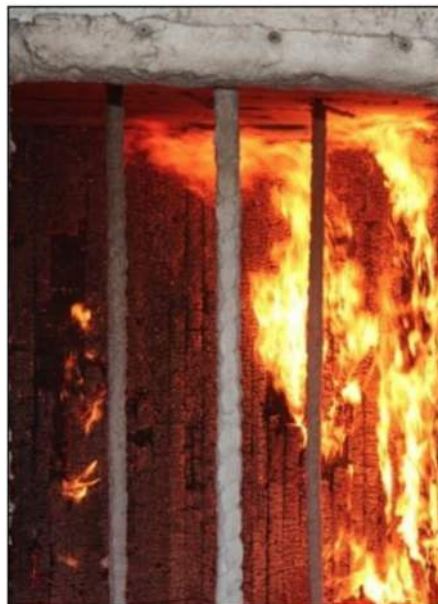
Reignition in the corner of the room leading to the second flashover
