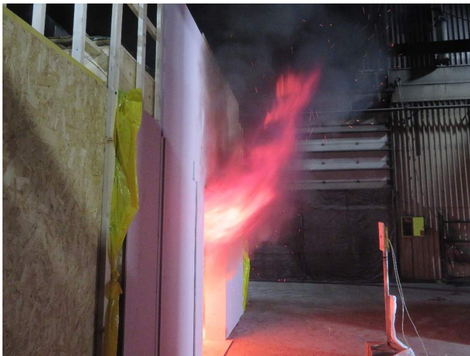
Figure 84 – Flames emerging following flashover
