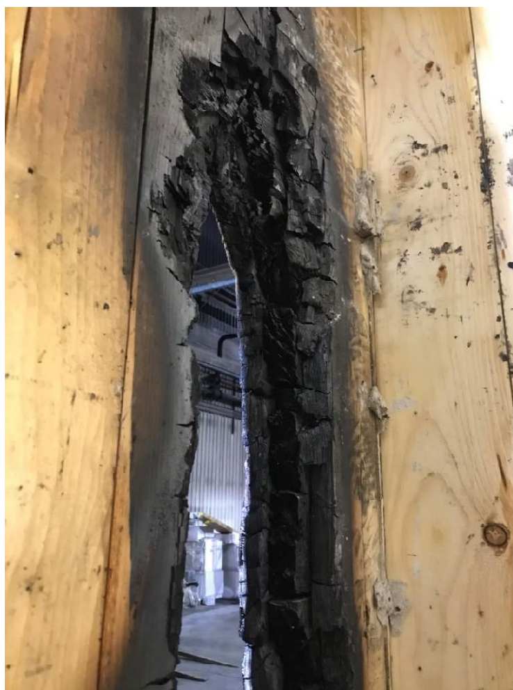
Figure 75 – Localised burn-through of CLT panel leading to visible flaming on the outer surface
