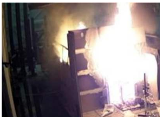
Test 1-6 – integrity failure at 160 minutes followed by termination
