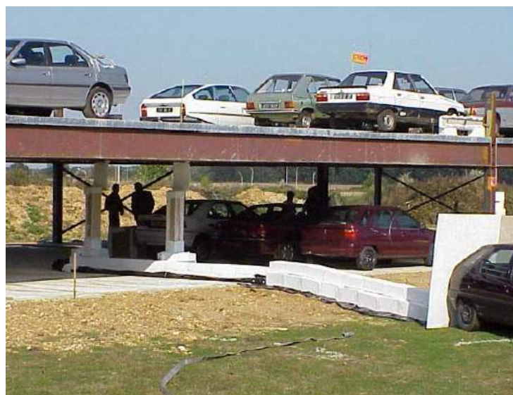
Figure 7 – The open car park configuration used in the tests sponsored by ECSC 14 . This is for the setup in test 2.
