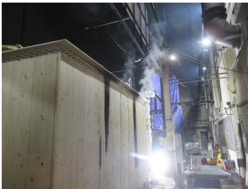
Figure 49 – Smouldering combustion through the back wall
