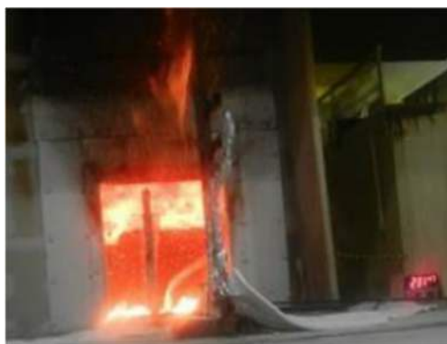
Test 1-4 – second flashover at 151 min followed by termination
