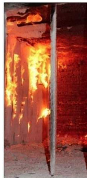
Flames escaping through the joints of the last protective layer
