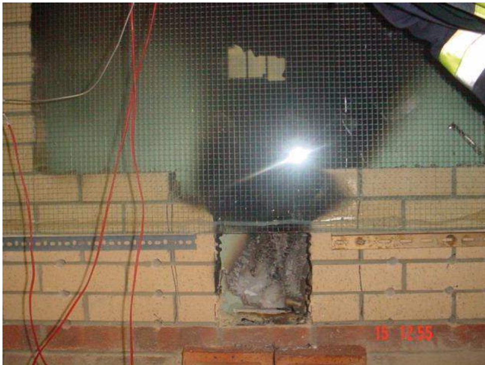
Figure 14 – Localised damage to “reverse” wall construction
