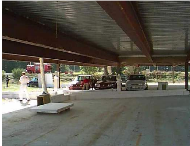
Figure 5 – The open car park configuration used in the tests sponsored by ECSC 14 . This is for the setup in test 1.
