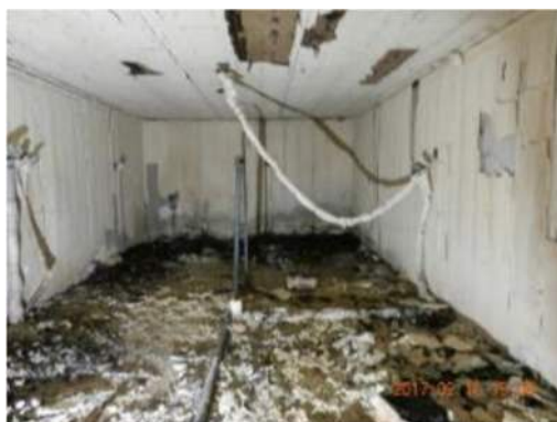
Test 1-1 – gypsum boards remained: 2 layers on the ceiling and 3 layers on the walls
