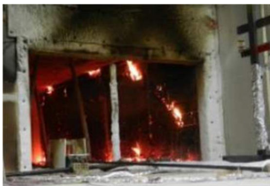
Test 1-3 – gypsum boards remained: 2 layers on the ceiling and 2 layers on the walls (W3 and W4)
