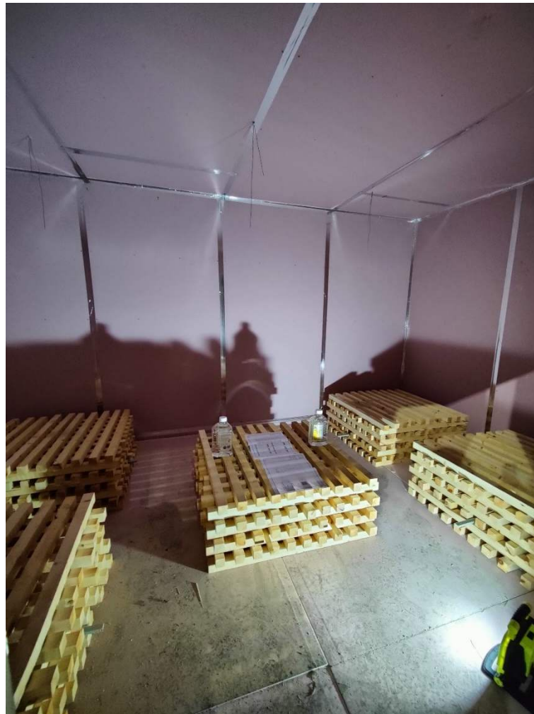
Figure 2 – Internal view of the fire compartment showing the layout of the fire load
