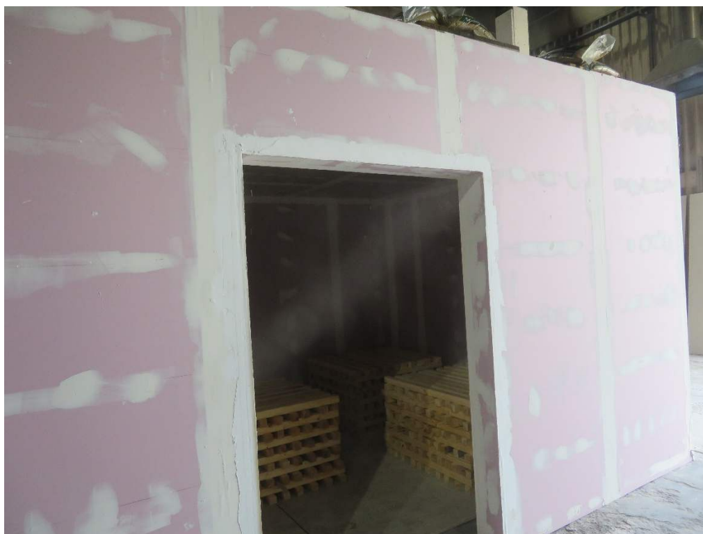
Figure 59 – Front of compartment prior to ignition showing single ventilation opening
