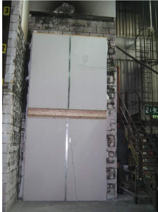
Figure 26 – “Interior” view showing plasterboard to timber frames and central beam
