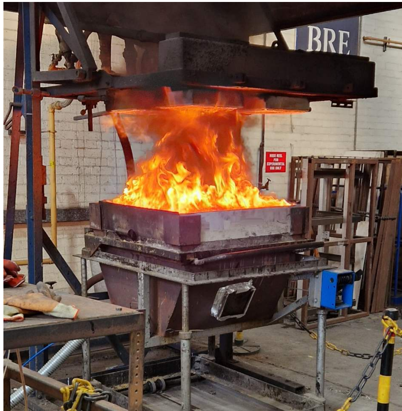
Figure 10 – A fire penetration roof test, with the flame plume having risen just above the surface combustion heaters (see left pair). Some samples tested result in taller flame plumes. Note that the entire surface area is burning but this will not be included in the report as it is not a reportable characteristic.
