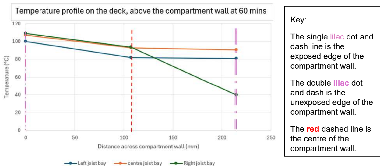
Figure 36 – Temperature profiles on the deck of the composite board created from data without the need to correct for ambient air temperature since the temperatures at the centreline and unexposed edge were all less than 140°C
