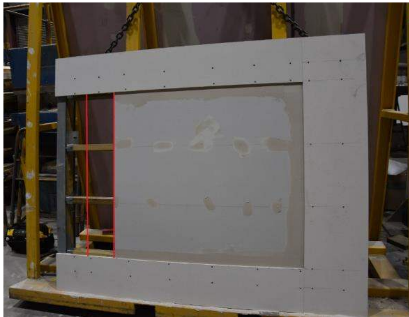
Figure 11 – A roof sample laid on its side showing the calcium silicate boarded perimeter and the plasterboard 'ceiling' in the centre.
