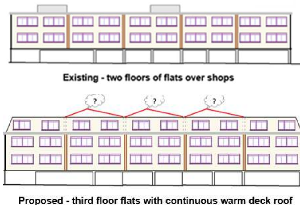
Figure 3 – A typical development opportunity where the building (after the work is complete) would remain less than 15 m tall and therefore the guidance at b., in Figure 1 above, would apply
