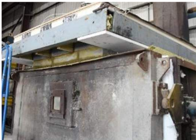
Figure 5 – A photograph of a sample undergoing installation onto the 1.5 m cube intermediate furnace
