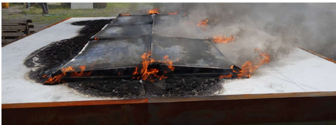
Figure 10. Experiment T3. The whole area underneath the PV array was affected by the fire.
