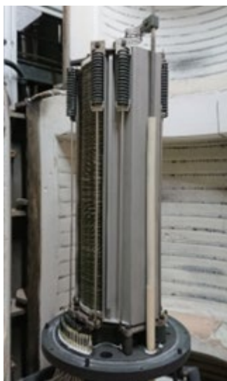
Figure 38 FCE's commercial stack in production test stand.
