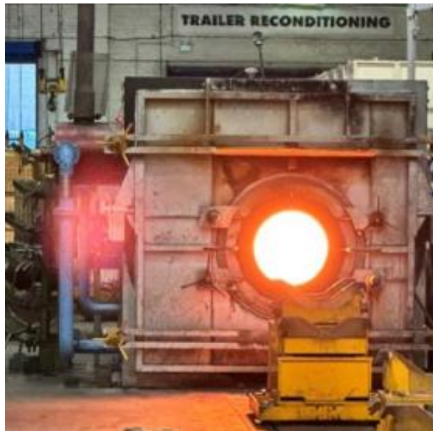
Figure 3: CSC furnace front view, showing forging hole in the centre and burner/flue gas exit to top left (in red)
