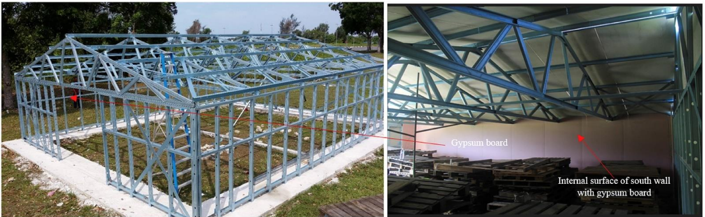
Figure 24. LSF building experiment using a natural fire (original from [47]).
