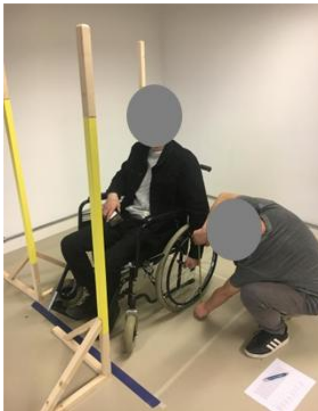
Figure 57. Example of straight down reach - no trunk movement (vertical height) measurement being taken by LU research team.
