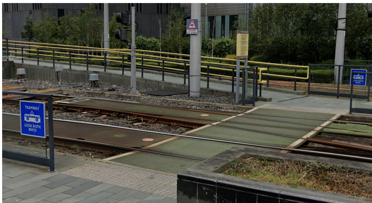
Figure 12: A crossing on Manchester Metrolink, with tactile paving, low signage and distinct colours (courtesy of Google).
