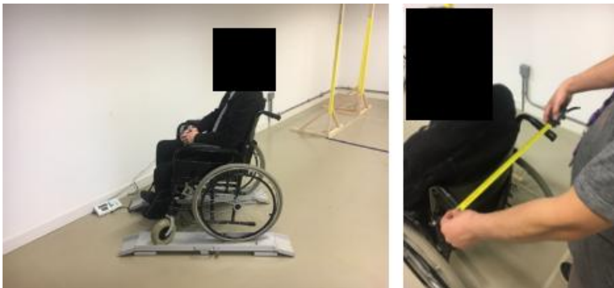
Figure 38. LU research team demonstrating measurement of combined weight of occupant and their mobility aid (left image) and distance between the wheeled mobility aid handles (right image).
