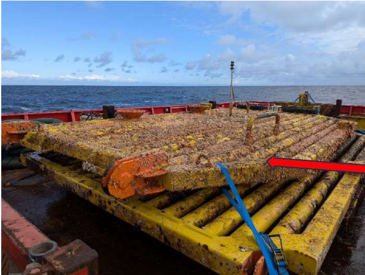
Photograph 8-1: Water injection wellhead protection structure hatch (I2) (depicted by red arrow) on top of one of the Type 1 template protection structure hatches
