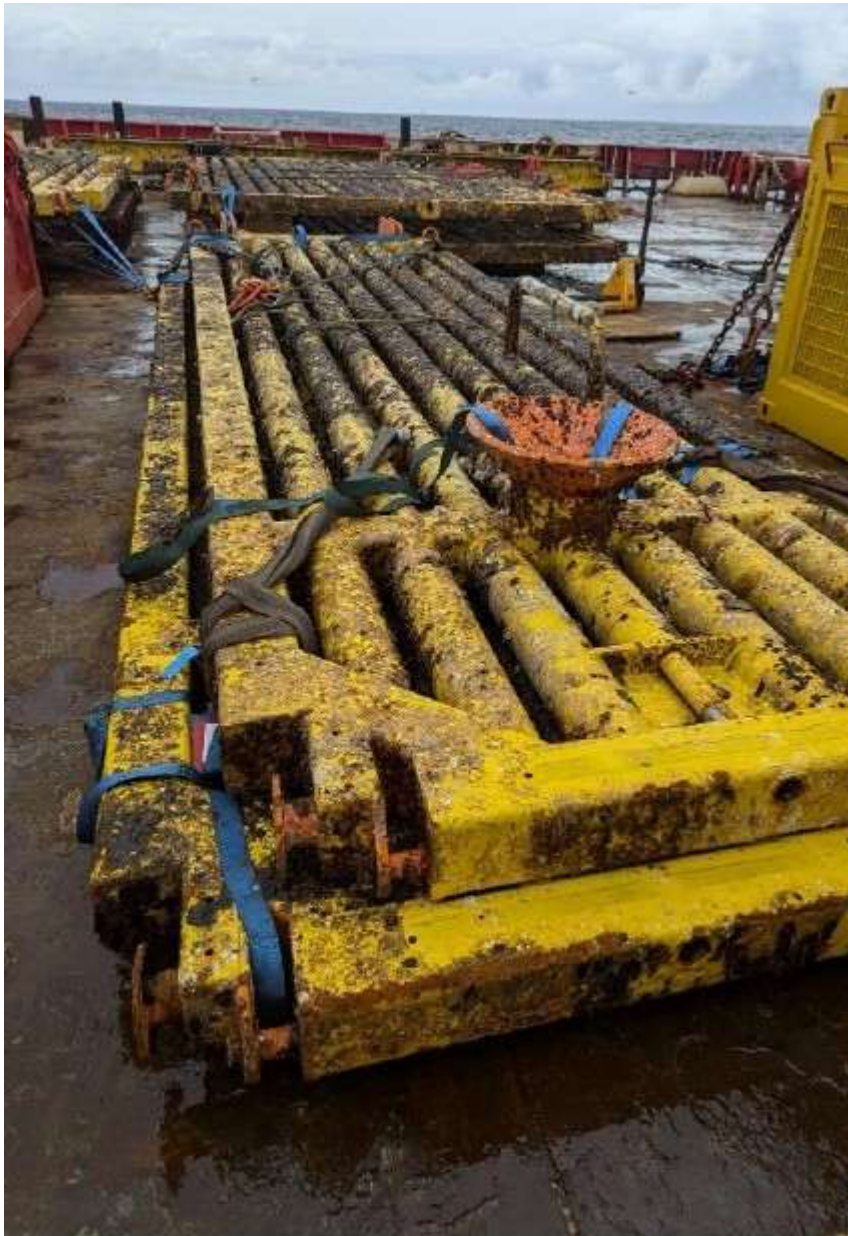
Photograph 8-3: One of the Type 2 template protection structure hatches
