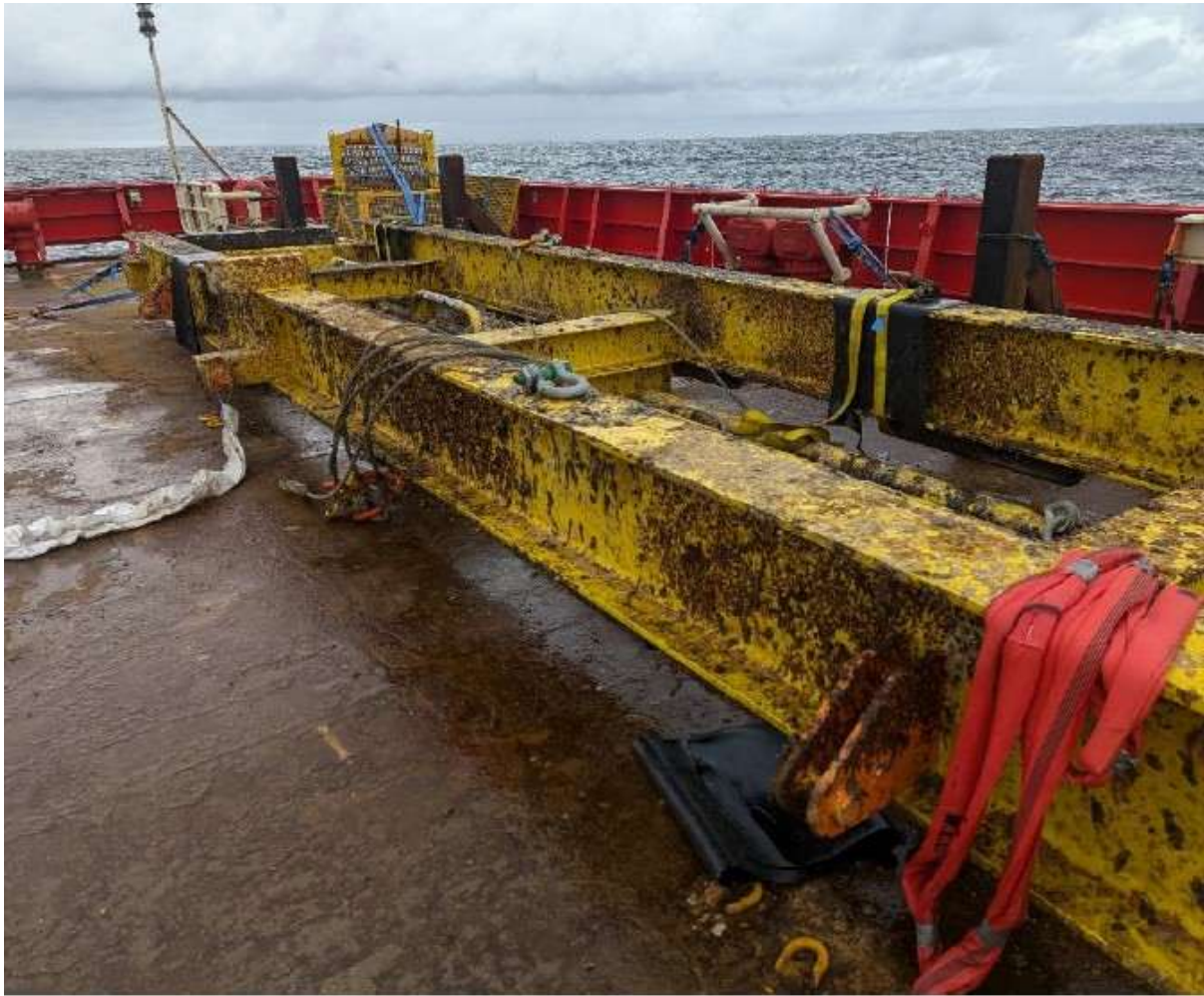
Photograph 8-4: The Type 3 template protection structure hatch
