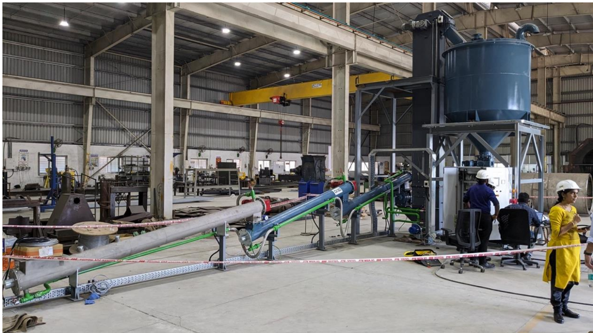
Figure 2.3.2. Assembly of the char cooling conveyors in Anergy's factory
