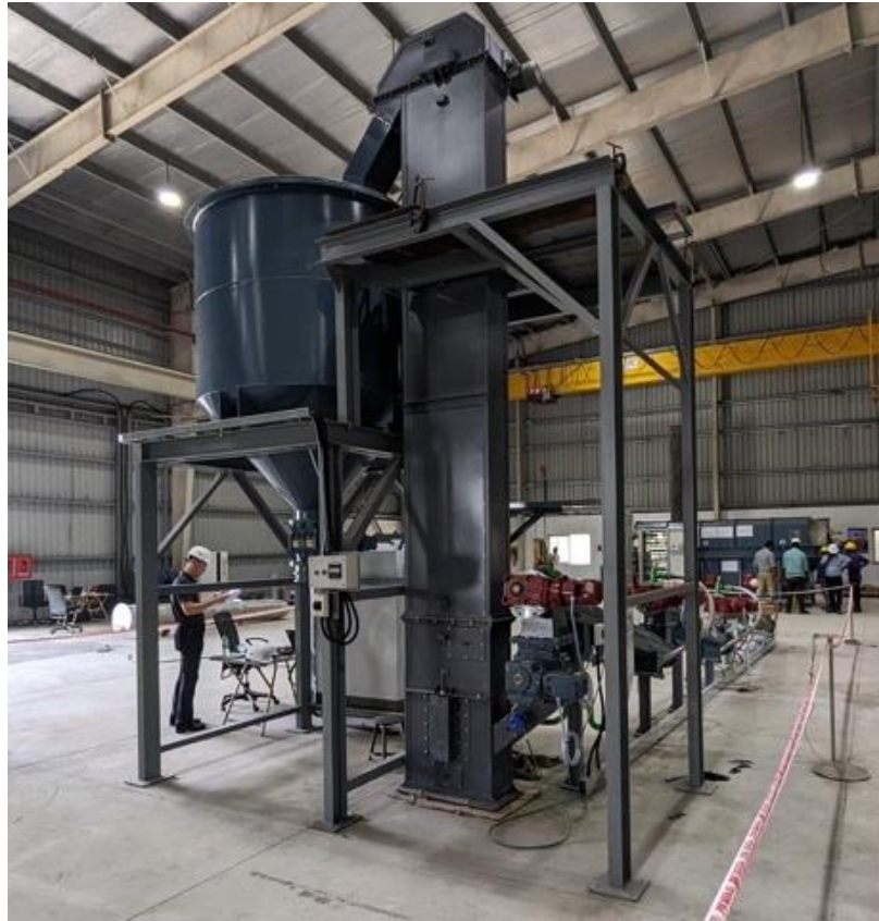
Figure 2.2.2.2. Char bin trial assembly in Anergy's factory in Chennai, India
