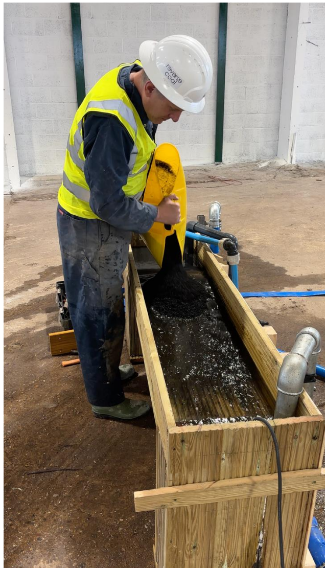
Figure 2.1.9. Biochar pumping trials highlighting flowing waterbed method
