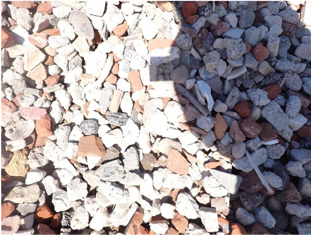
Photograph 5 – Aggregate containing a battery on 17/09/2024
