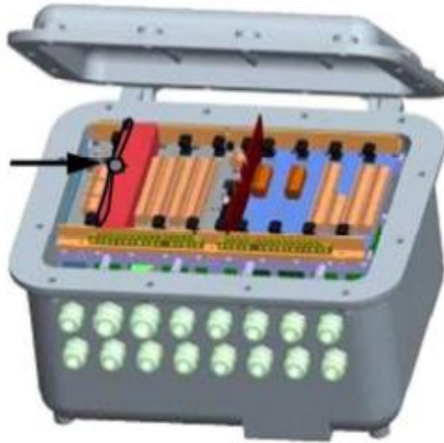
Figure 4 Sealing of basic modules
