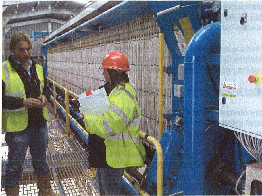
Photograph 14 - The presses squeeze out the water and the clay drops to the ground. A full cycle takes approximately 30-40 minutes.
