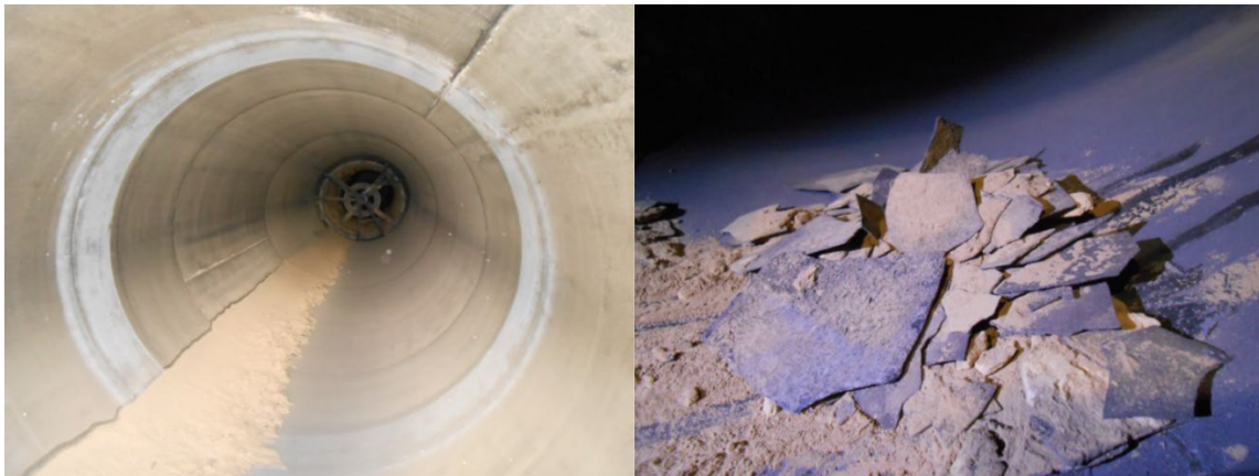
Figure 17: Left: View inside the kiln tube after the trial. Right: Detailed view on the shards forming the layer on the kiln tube wall.
