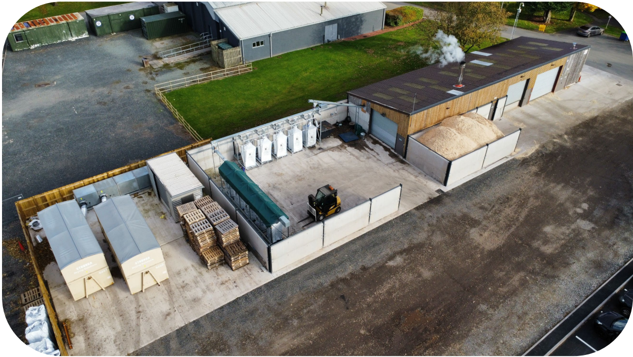
Figure 3 – A.W. Jenkinson Newton Rigg site showcasing BBB's Biomacon C500-I pyrolysis unit, peripheral equipment, pre-existing building and container dryers.
