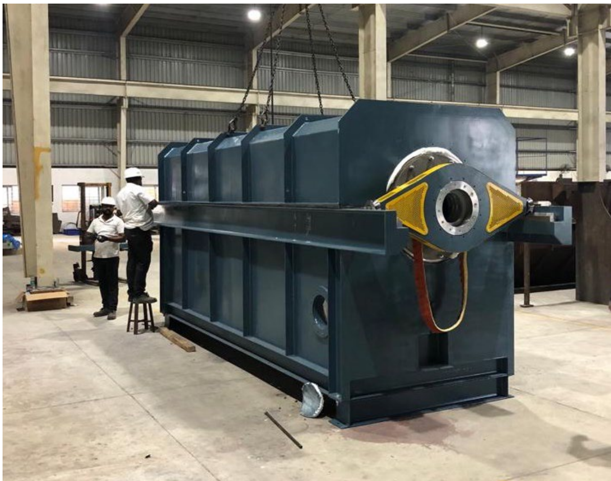
Figure 2.2.2.1. HTP Kiln being manufactured in Anergy's factory in Chennai, India
