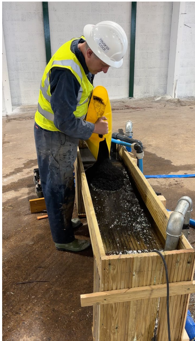
Figure 2.1.9. Biochar pumping trials highlighting flowing waterbed method
