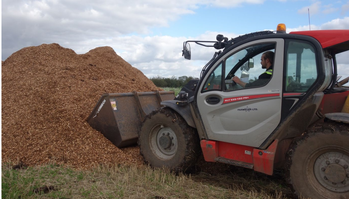
Figure 4.2.2. Lapwing operators using a telehandler to handle and pile woodchip
