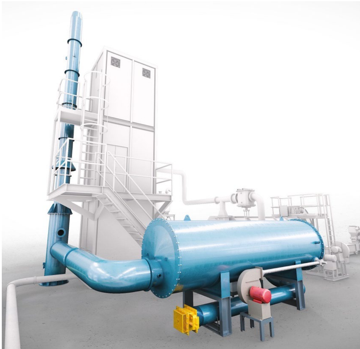
Figure 2.1.6. 3D Visualisation of Combustor and Plant Exhaust (credit: Bilfinger UK)
