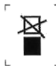
IBCs NOT capable of being stacked
