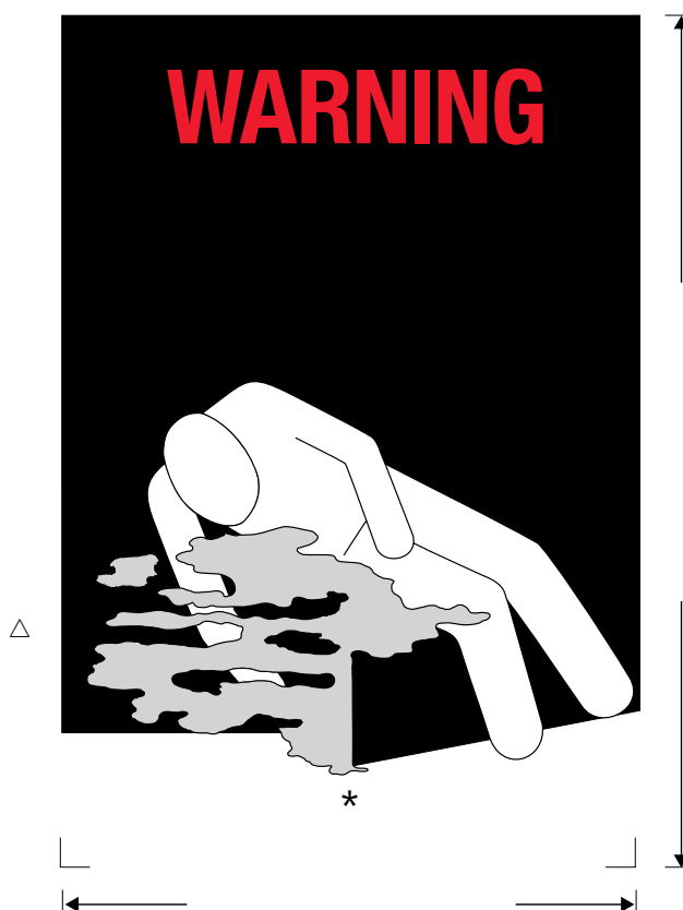
△ Asphyxiation warning mark for cargo transport units
