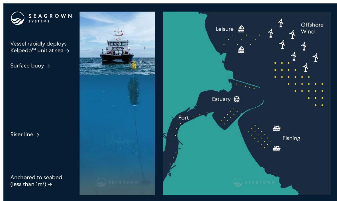
Figure 3. Left: SeaGrown vessel Bright Blue deploys Kelpedo at sea, with cutaway image showing anchor, riser line, Kelpedo and surface buoy. Right: Examples of use cases of Kelpedo including ports, estuaries, co-existence with fishing and leisure, and co-location with the offshore wind industry.
