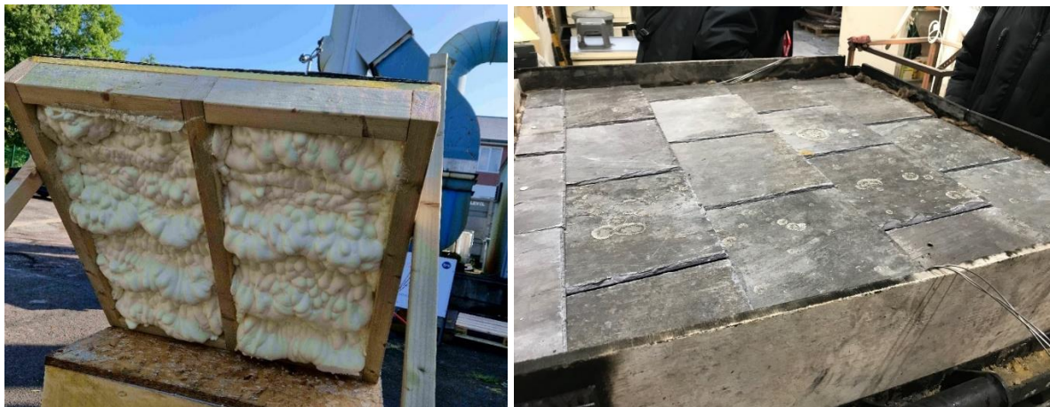
Figure 3. Underside of very old slate without sarking (Sample C)
