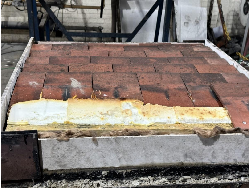
Figure 8. Discolouration of insulation below clay tiles (sample A)
