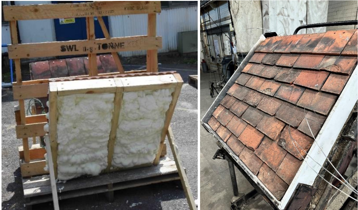
Figure 2. Very old plain clay with sarking (Sample B)
