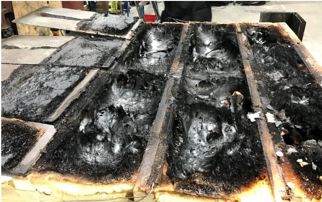
Figure 9. Smouldered insulation below the slate tiles (Sample C)
