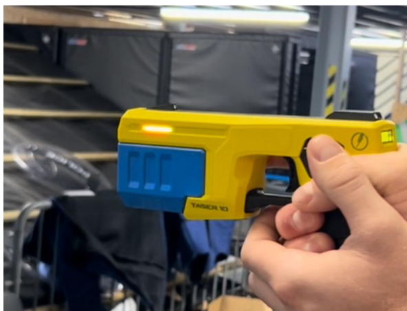
Figure 47, T10 with HALT magazine fitted showing yellow sidelight
