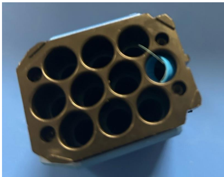
Figure 51, HALT magazine and detached cartridge 'collar'
