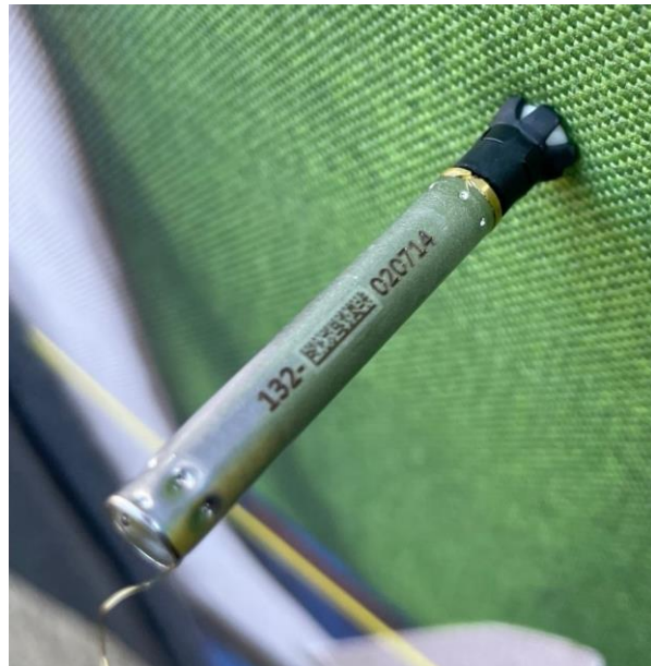
Figure 18, Taser 10 probe with compressed impact absorber
