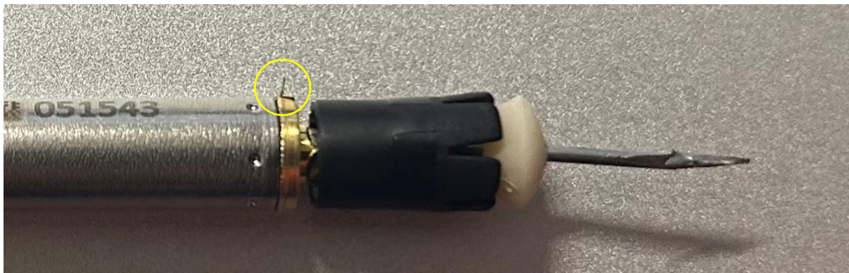
Figure 45, probe body with wire protruding, fired from 10m
