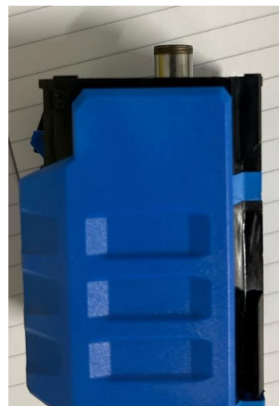
Figure 50, HALT cartridge jammed in magazine
