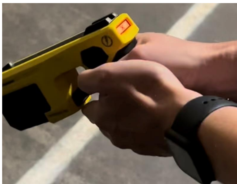
Figure 39, device T2 exhibiting 'critical error' warning
