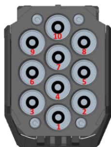
Figure 87, cartridge rear view showing bore numbering system, © AXON Inc.
