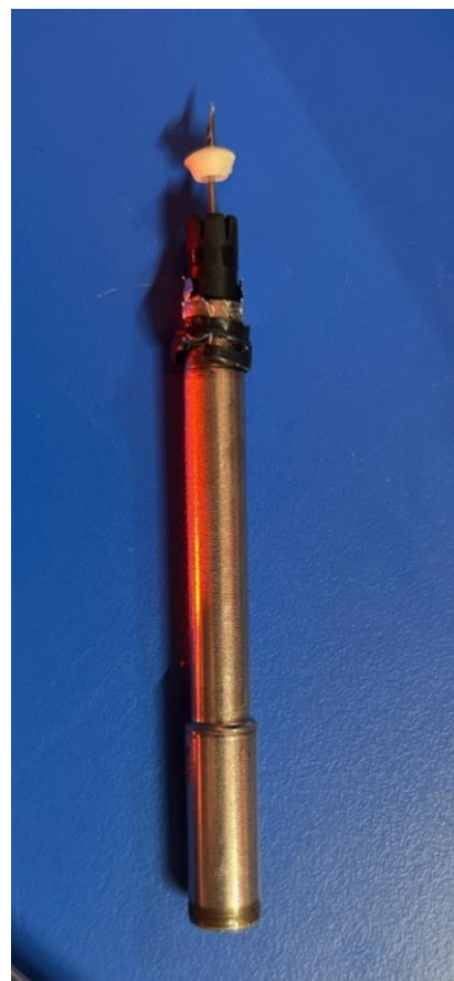
Figure 75, misfire cartridge removed from magazine
