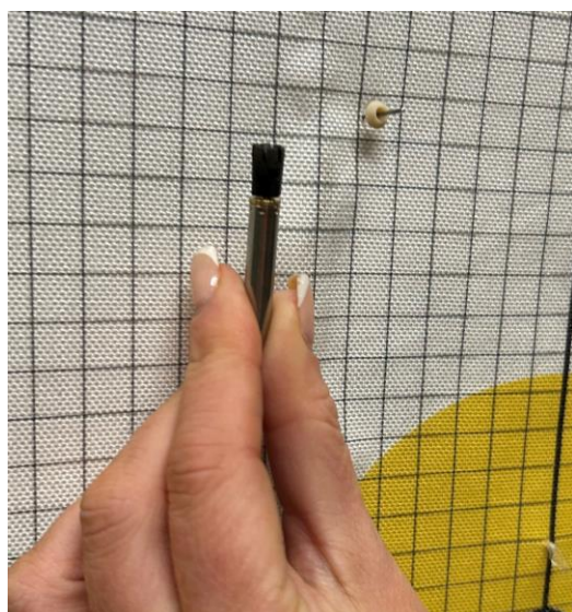
Figure 46, dart separated from probe body
