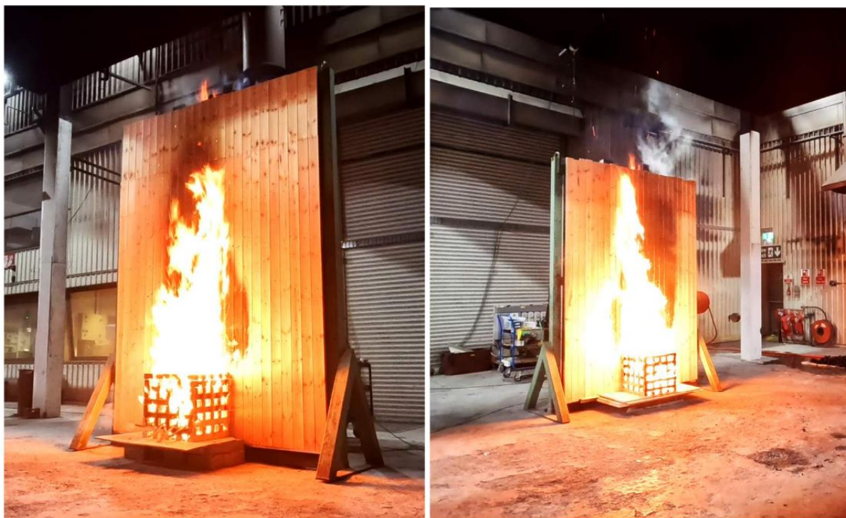
Figure 16. Fire penetration through samples (left) CD-Virgin-9mm after ca. 6.5 min, (right) PS-Virgin-19mm after ca. 12 min)
