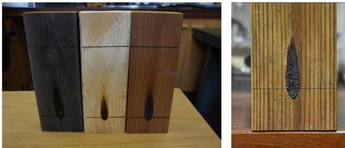
Figure 5. Samples following small flame test, from left to right: PS-TM-Aged, PS-Virgin, PS-TM-New and PS-TM-FR
