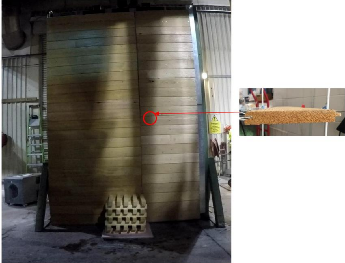
Figure 18. 19 mm thick Cedar timber cladding (CD-Virgin-19mm) installed on the intermediate-scale rig
