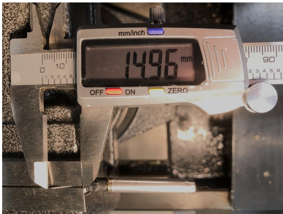
Figure 18: Compression testing of the impact absorber of a T10 probe, showing an exposed dart length of approximately 15mm after compression (compared to 11mm without compression).
