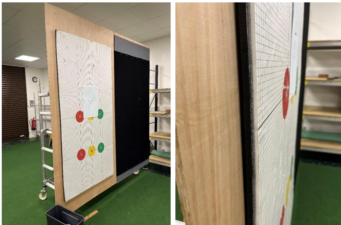
Figure 53: The target used for kinetic testing – an Axon-provided flat layered target mounted to a plywood backing for support. Left: The target with graph paper overlayed for POI measurements. Right: A close-up of the side of the target.
