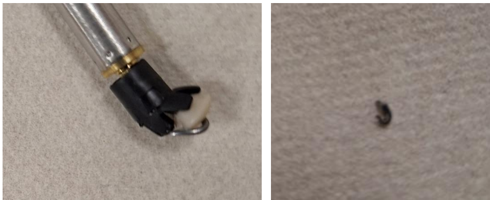
Figure 20: Photos of the T10 dart after shot 736, in which a fragment of the dart remained in the model. Left: The T10 probe; note the missing end of the dart. Right: Snapped piece of dart removed from bone.
