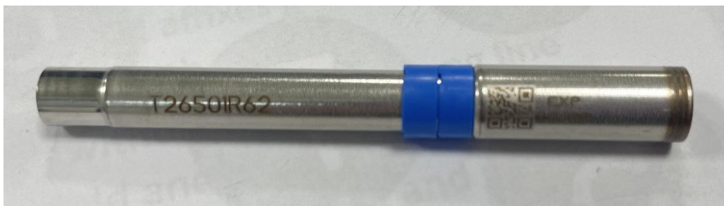
Figure 46: A HALT cartridge with two blue ID bands, preventing it being loaded into a magazine bay.
