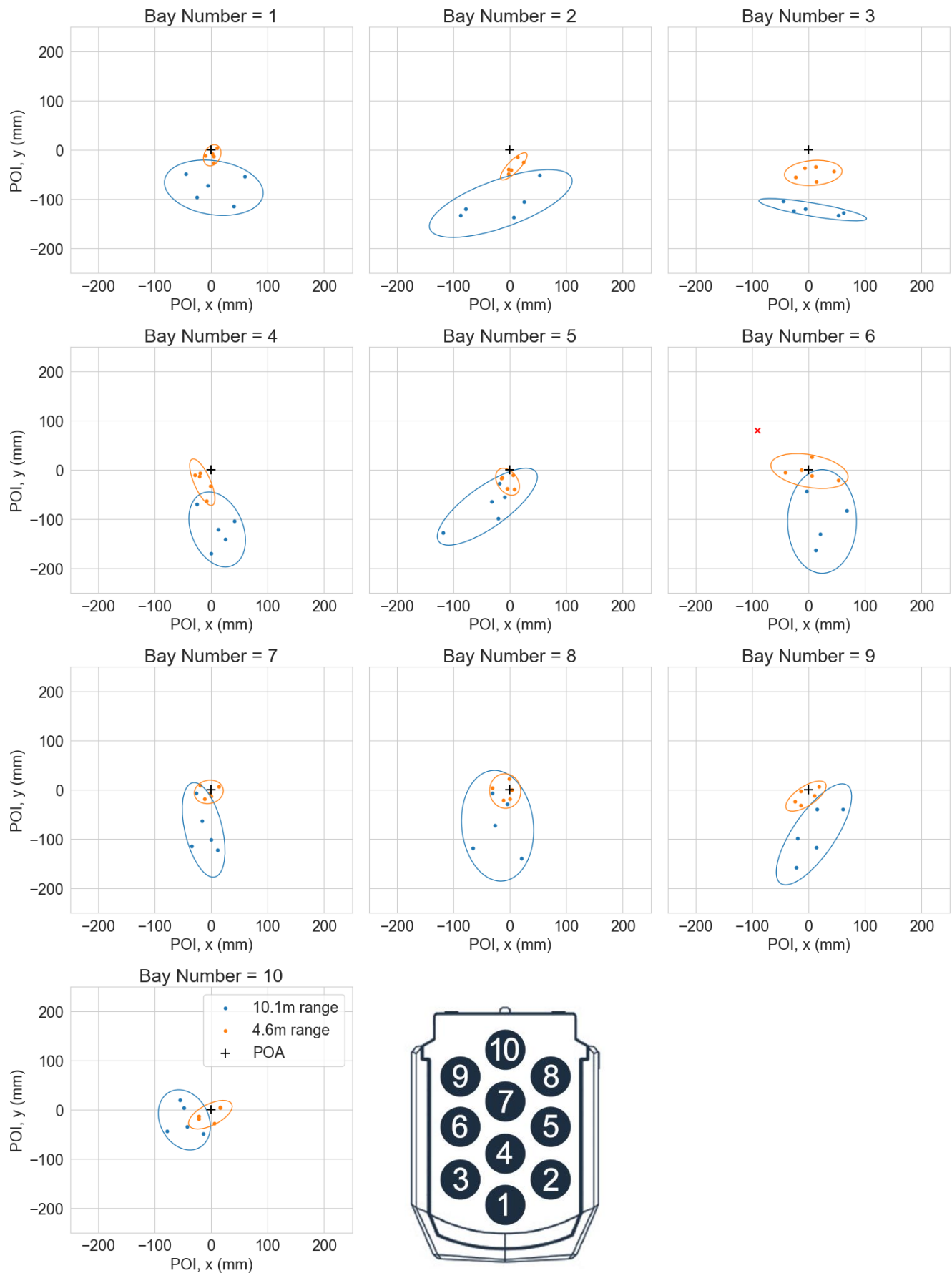
Figure 3: Plots of POI data by bay for duty cartridges in magazine S1 at a range of 10.1m (blue) and 4.6m (orange). The black cross indicates the POA, the points are the raw POIs, the red cross is an outlier point at 10.1m excluded from the analysis (the same as in Figure 2), and the ellipses are confidence ellipses that correspond to containing 95% of the data. A diagram of the bays (from the rear of the device – i.e. the position of an operator) is provided for reference.
