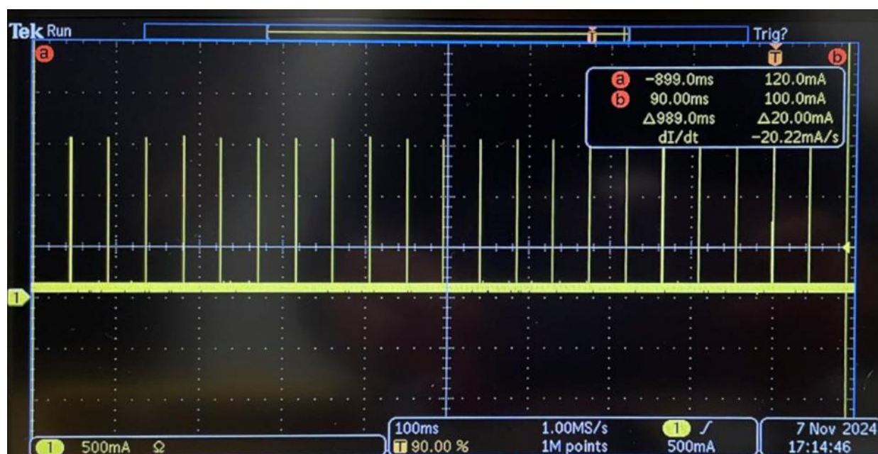
Figure 28: Typical waveform output during Axon-specified testing, showing the train of electrical pulses. The span of the x-axis is 1000ms.
