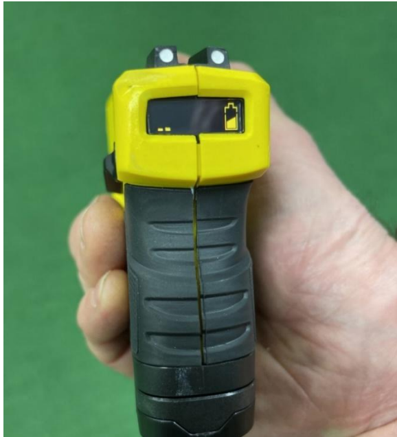
Figure 23: Slight separation/displacement of the frame after drop onto the front top corner of the device (position 10). The magazine was ejected on this drop and was replaced manually in the right-hand picture to show the frame displacement.
