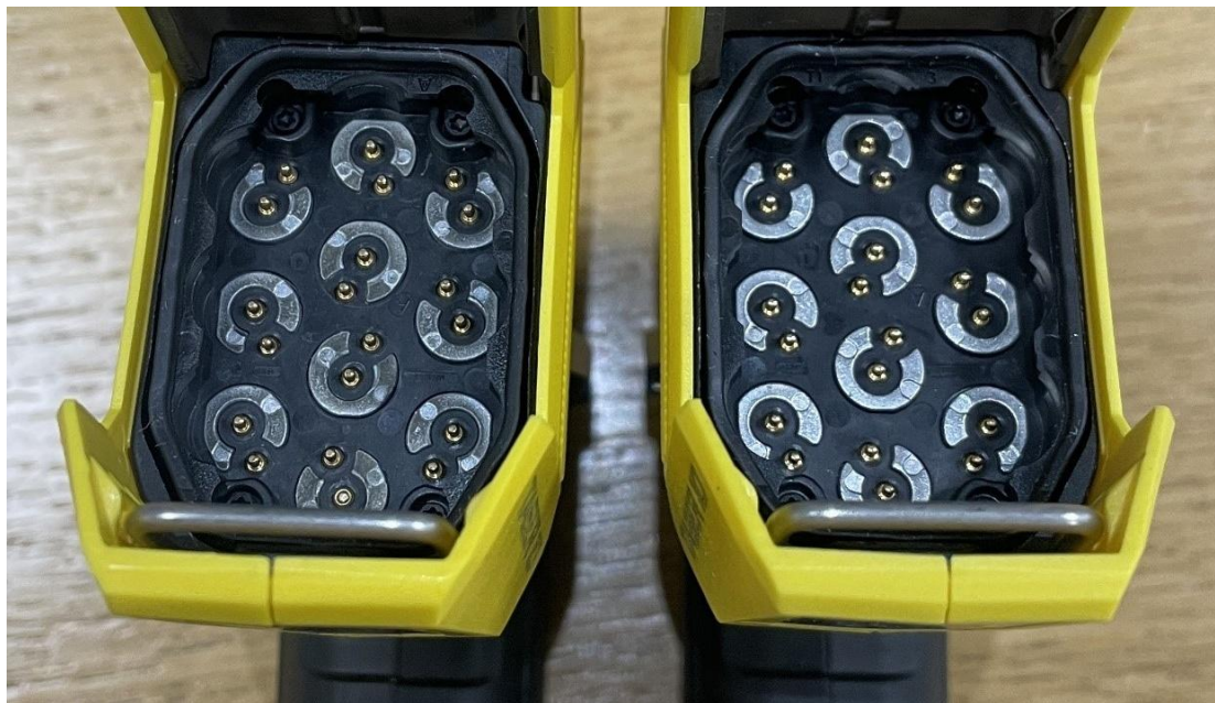
Figure 49: A comparison of a heavily used interposer bucket (left; over 310 shots, and the same interposer bucket as in Figure 48) and an unused interposer bucket (right).
