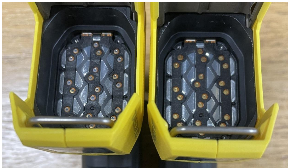
Figure 50: A comparison of a heavily used handle with the interposer bucket removed (left; over 310 shots, and the same handle as in Figure 48) and an unused handle (right), again with the interposer bucket removed.
