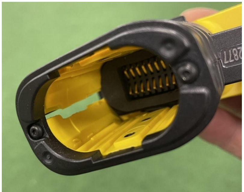
Figure 24: Separation/displacement of the frame after drop onto the left-hand side (position 6). The battery was ejected on this drop.
