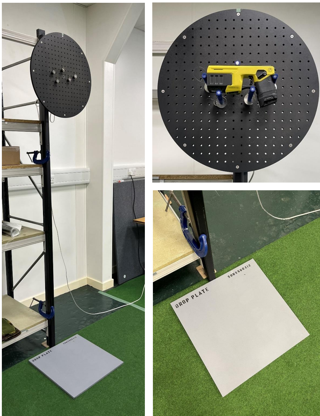
Figure 58: The drop rig developed in-house for drop testing. Left: the full 2m rig. Top right: a device mounted in the POM fingers controlled by electromagnets. Bottom right: the steel drop plate.
