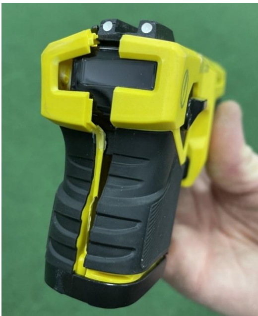
Figure 24: Separation/displacement of the frame after drop onto the left-hand side (position 6). The battery was ejected on this drop.
