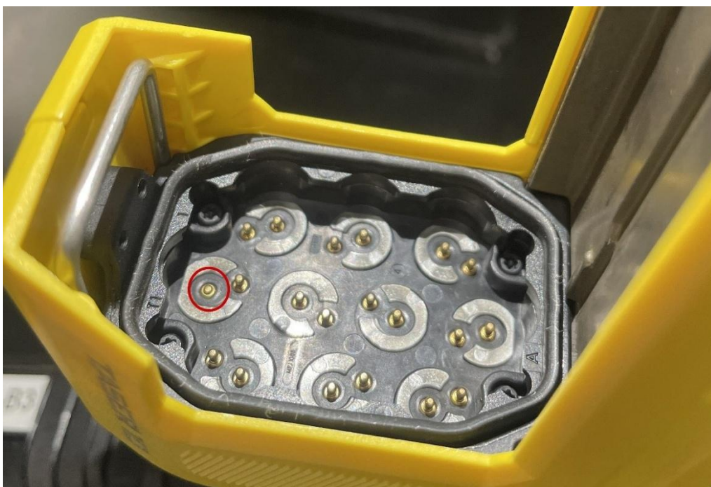
Figure 48: An interposer bucket with a permanently depressed pogo pin that could not be fixed (red circle).
