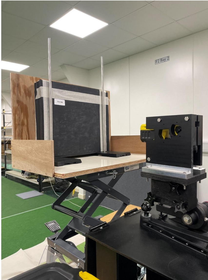
Figure 57: Setup of the skin penetration testing.
