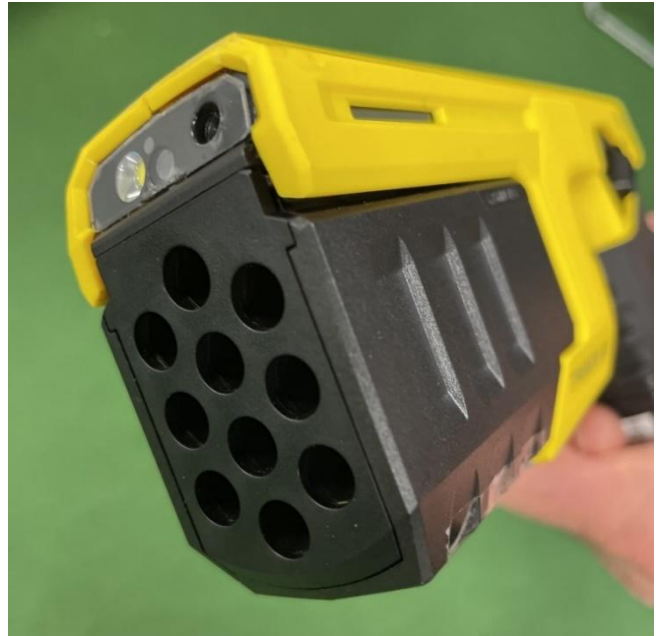
Figure 23: Slight separation/displacement of the frame after drop onto the front top corner of the device (position 10). The magazine was ejected on this drop and was replaced manually in the right-hand picture to show the frame displacement.
