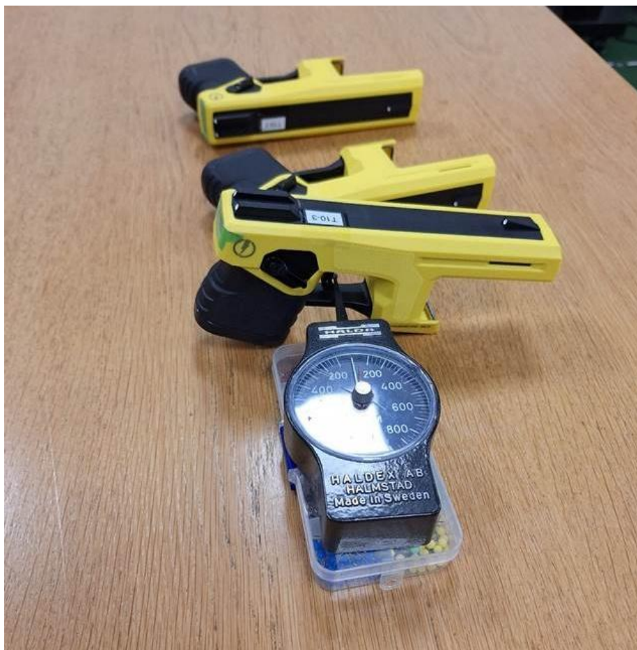
Figure 68: Testing setup for measuring the force required to pull the trigger for different handles with varying levels of use.
