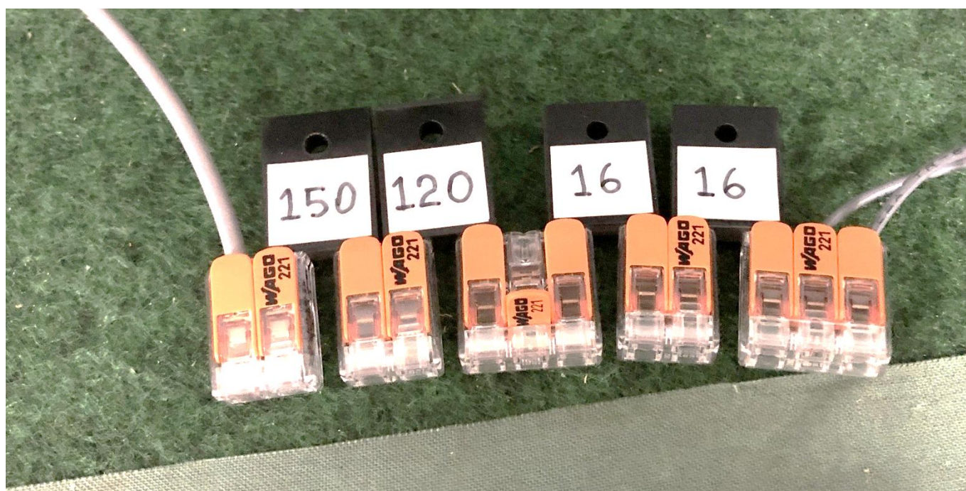
Figure 45: The resistor setup for one potential divider during Salvo 1.
