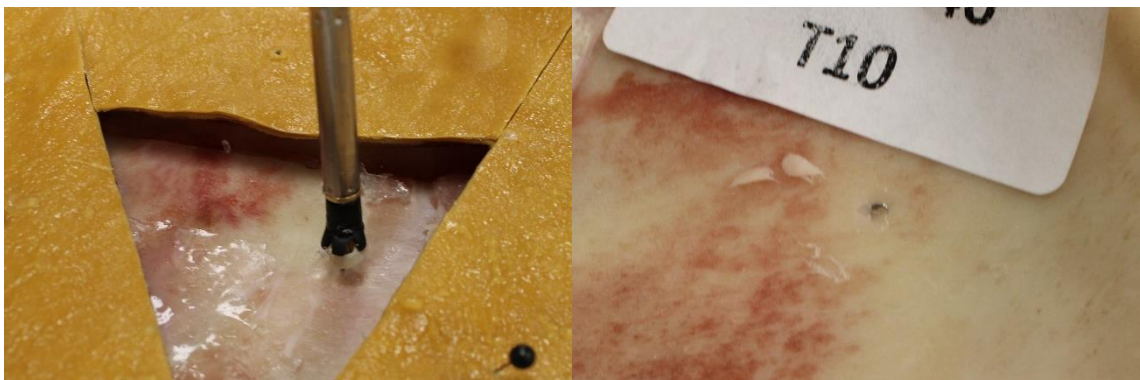
Figure 25: TASER 10™ probe embedded in skull surrogate. Normal side of model, showing probe embedded into bone ( left ). Internal face of the model, showing dart perforating through ( right ).
