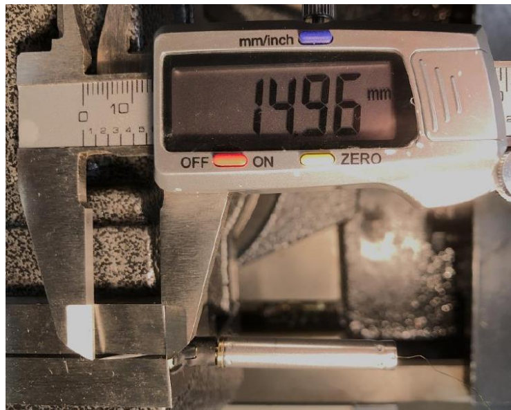
Figure 11. Length of dart after full compression of the probe's impact absorber.
