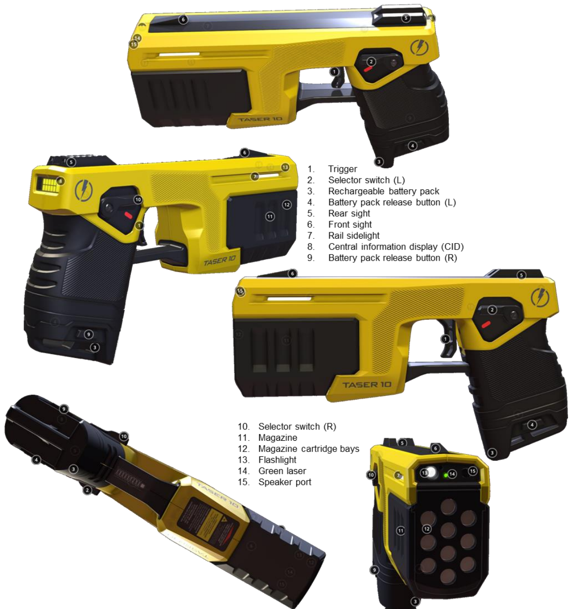
Figure 1. External features of the TASER 10™. Images are screenshots captured from a 3D model. 1
