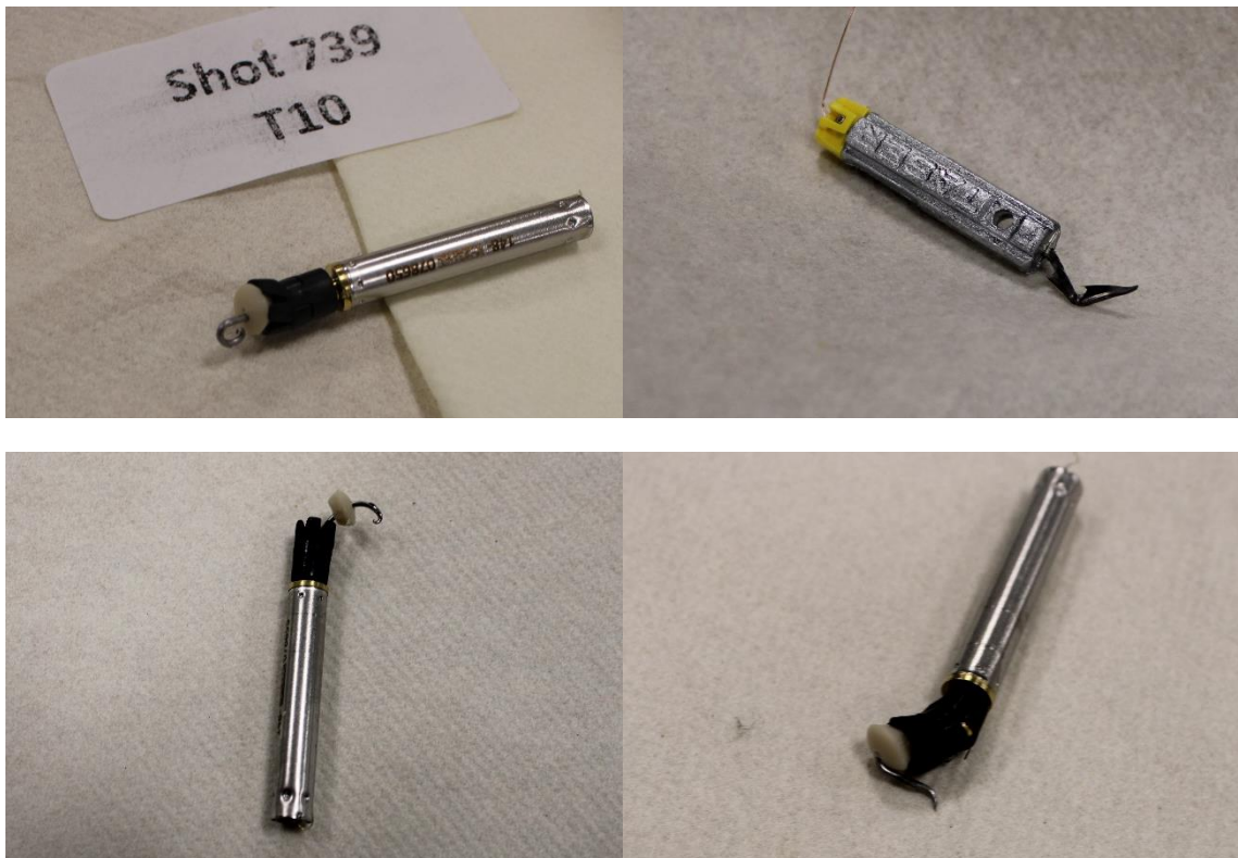
Figure 27: complex deformed shapes from skull surrogate fracture tests.
