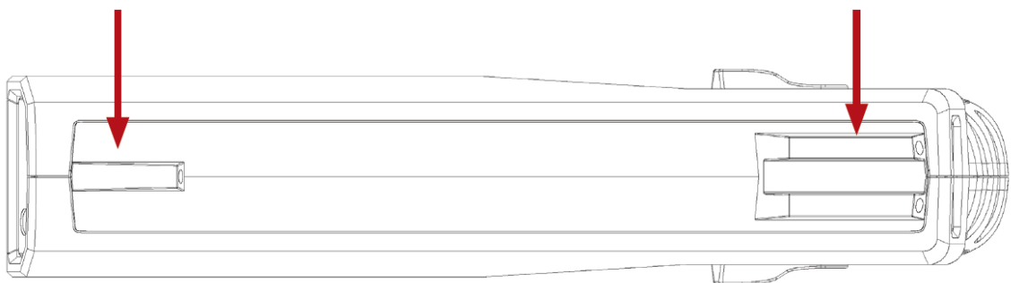
Figure 19: Location of mechanical sights on top of TASER 10™ body.
