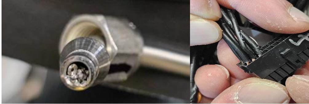
Figure 22. Examples of issues encountered during build: Swarf not cleaned out in hydrogen piping (left), and poor termination of connectors (right)
