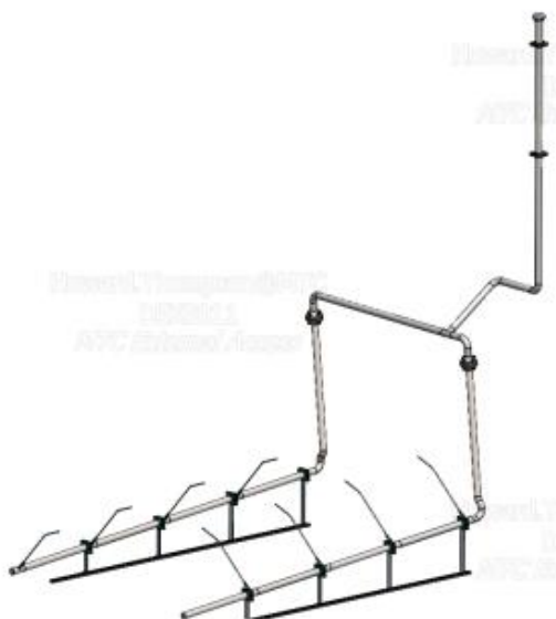
Figure 62: HiAB container venting system
