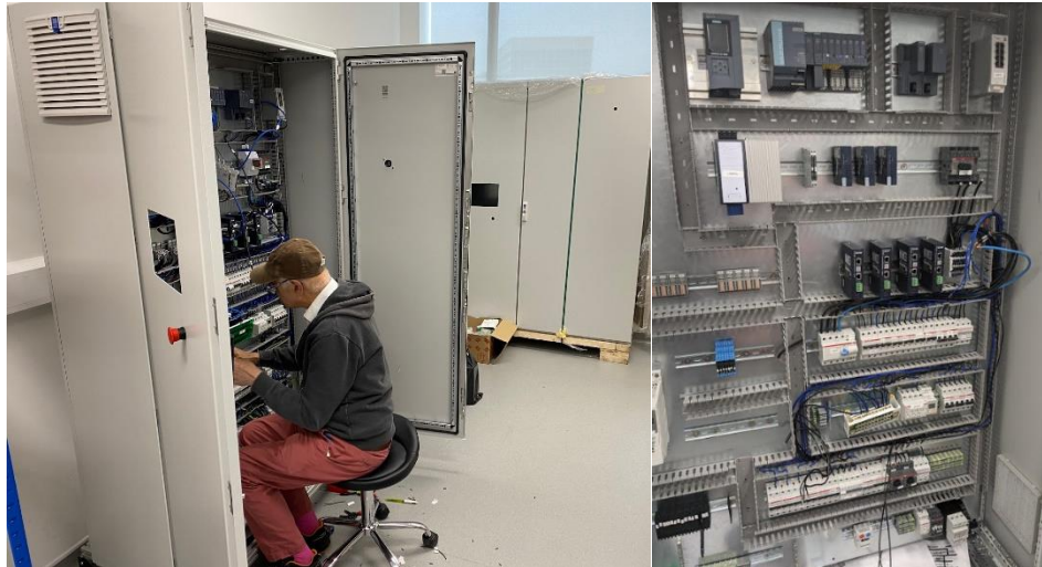
Figure 66: Electrical Panel Manufacturing at H2GO Power Facilities
