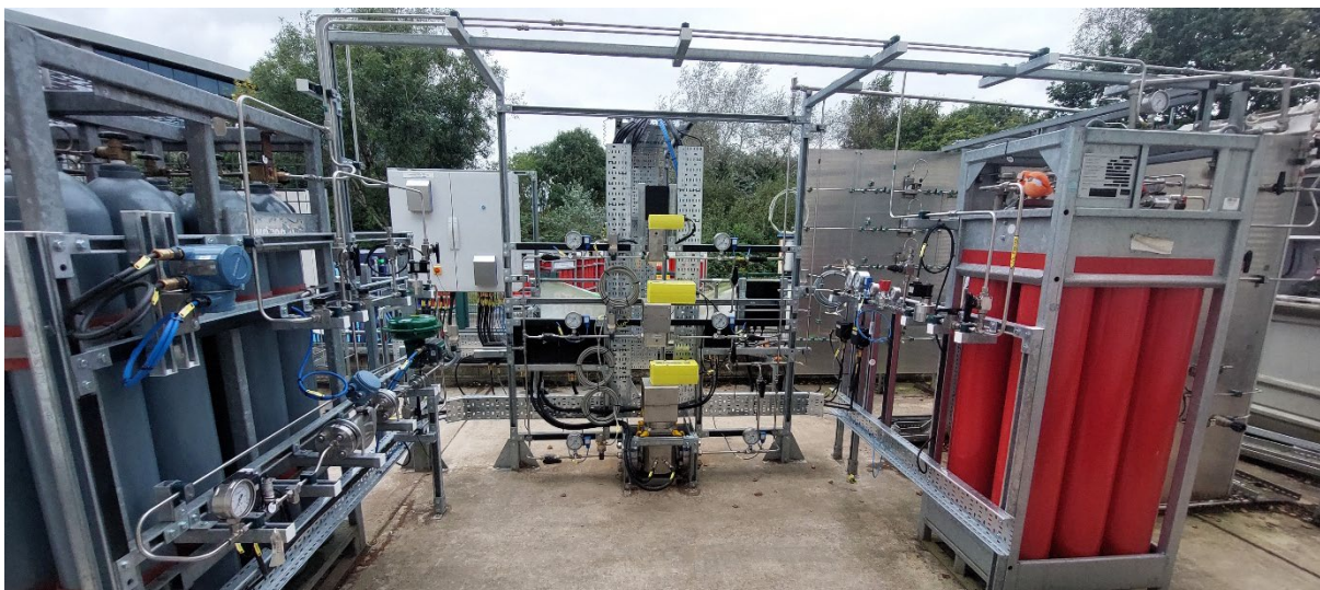
Figure 3: Flow loop at USW site with (left) low-pressure storage tanks, (centre) Dragonfly valves, (right) high-pressure storage tanks
