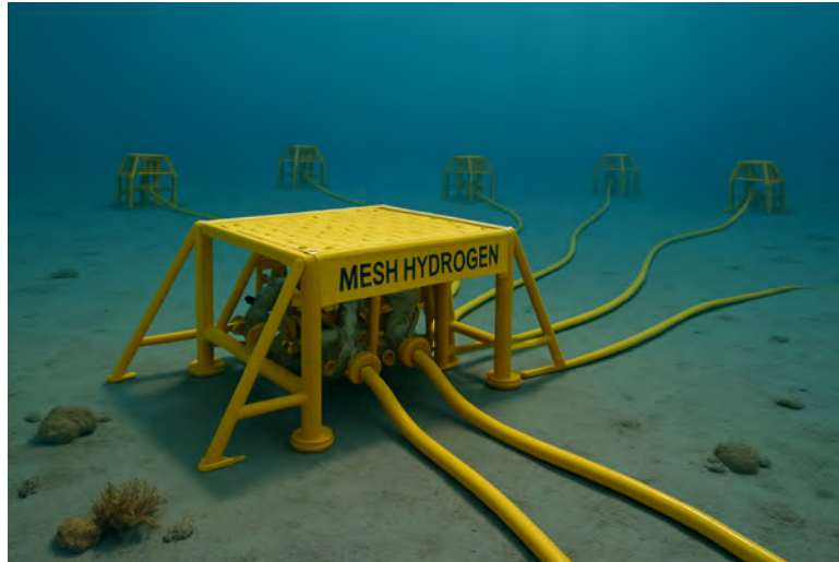
Figure 8: hydrogen storage subsea manifold and hydrogen wellheads
