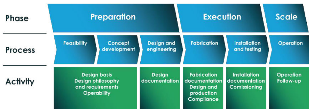
Figure 4-3: Process diagram realisation of an offshore or nearshore seaweed growing system (Agitec et al, 2023)
