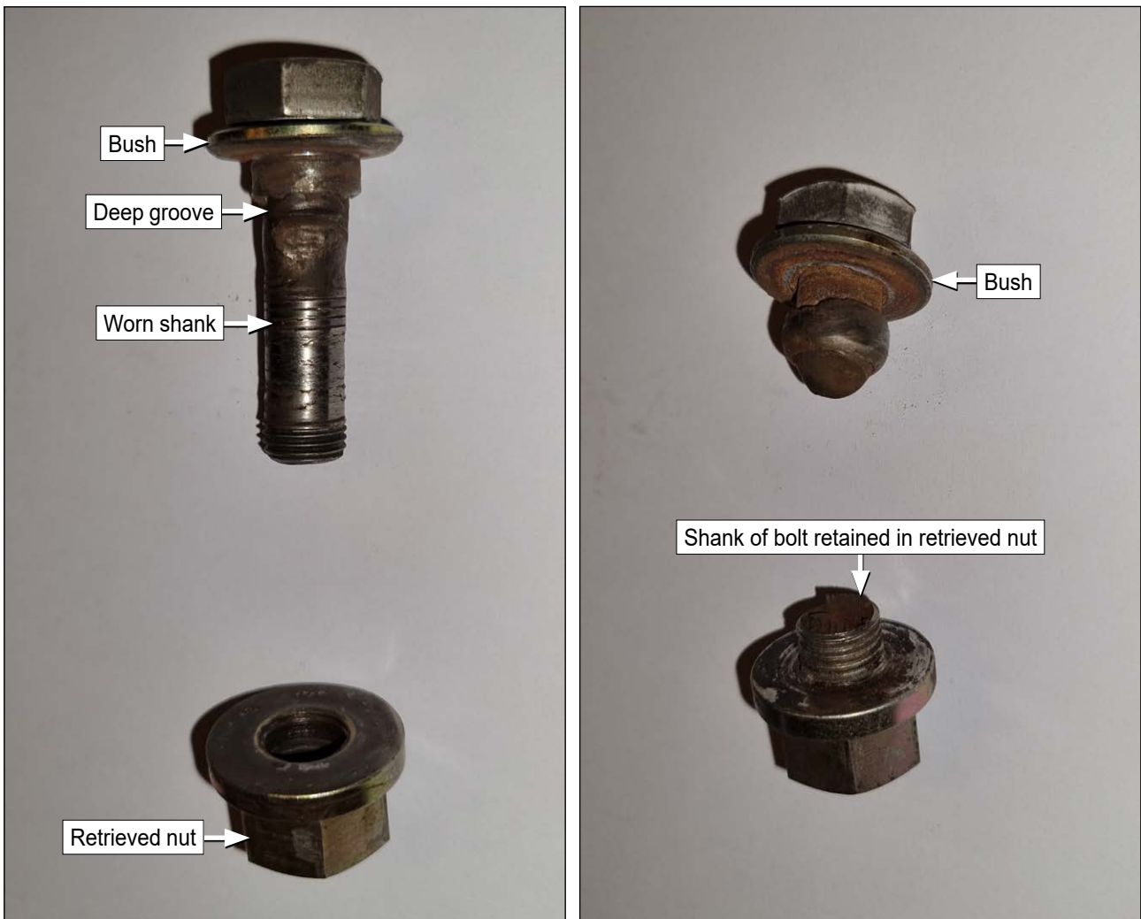
Figure 9: Damaged coupling drive bolts
