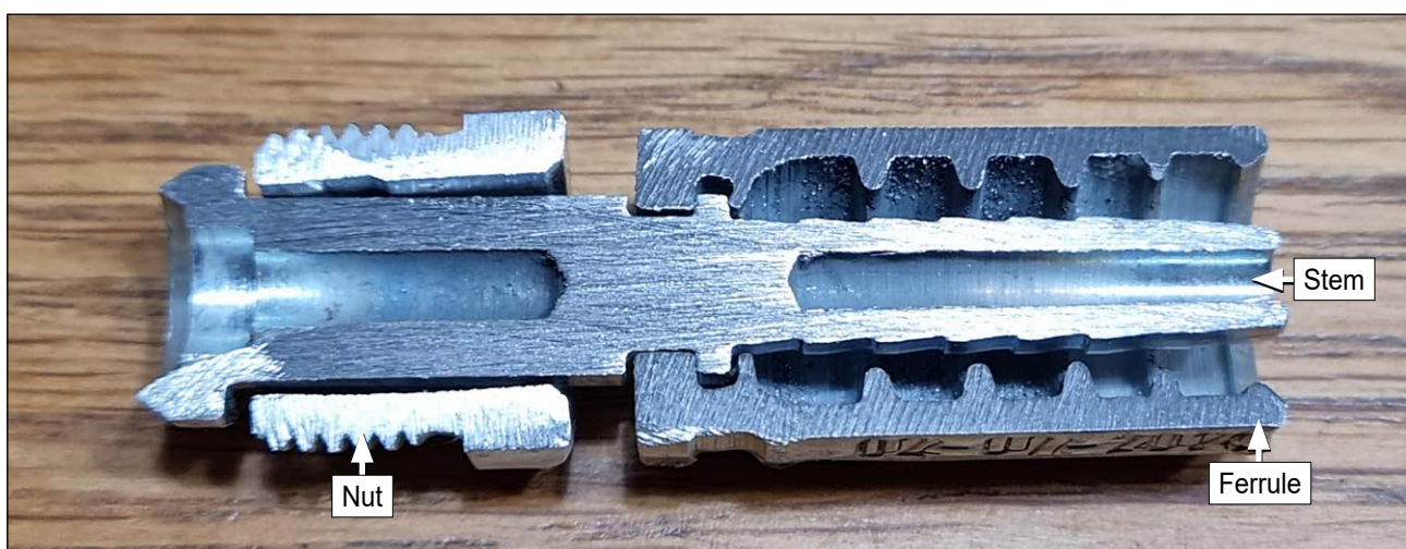
Figure 25: Section through flexible hose assembly coupling between cylinders C241 and C242
