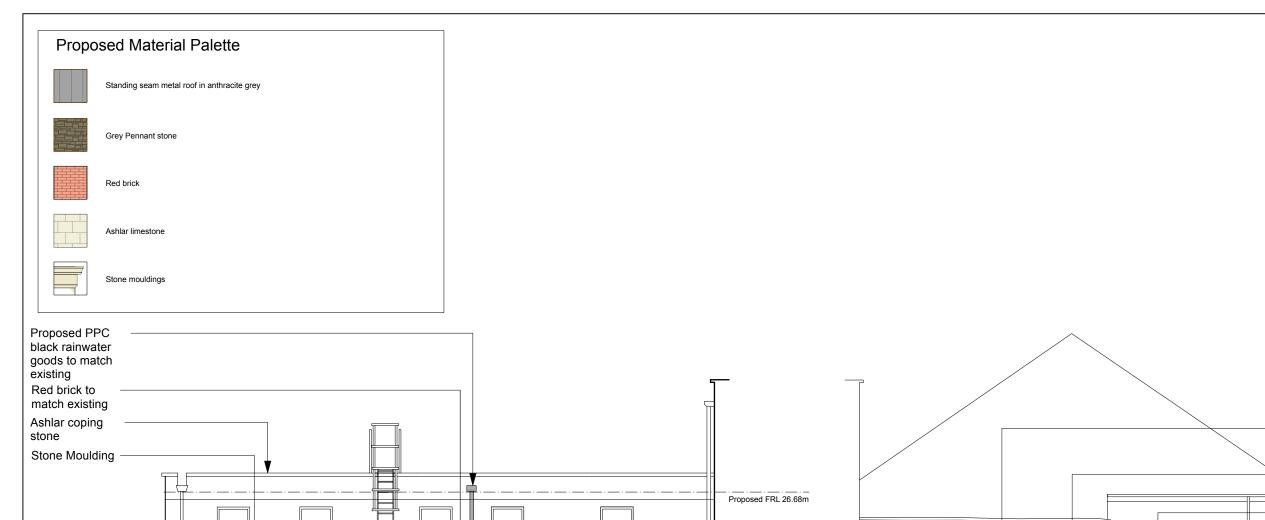
Antrhacite casement window Antrhacite glazed door Red brick wall to match existing PPC black rainwater goods Antrhacite casement window Proposed Upper FFL 23.68m Proposed FRL 23.40m Proposed GFL 20.68m proposed GFL 20.01m Courtyard North Elevation Courtyard South Elevation
