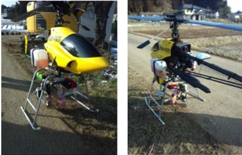
Figure 4: Robin-Pars remote controlled helicopter UAV (reproduced from Furutani et al., 2013).
