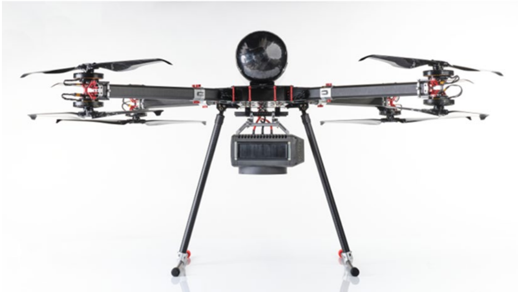
Figure 22: Hydrogen fuel cell and cylinder attached to a commercially available UAV (reproduced from Intelligent Energy, 2025).
