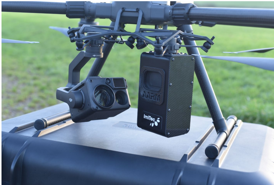
Figure 21: A DJI M300 UAV mounted with an Imitec AARM radiation monitor and a DJI H20t thermal camera (image supplied by the University of Bristol).
