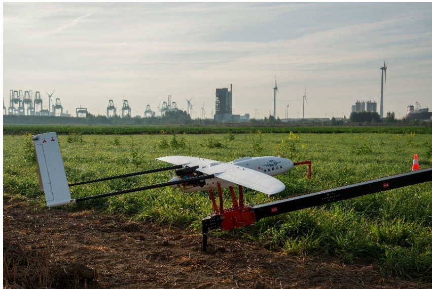
Figure 2: Penguin C fixed-wing UAV on launch catapult (reproduced from Geelen et al., 2022).
