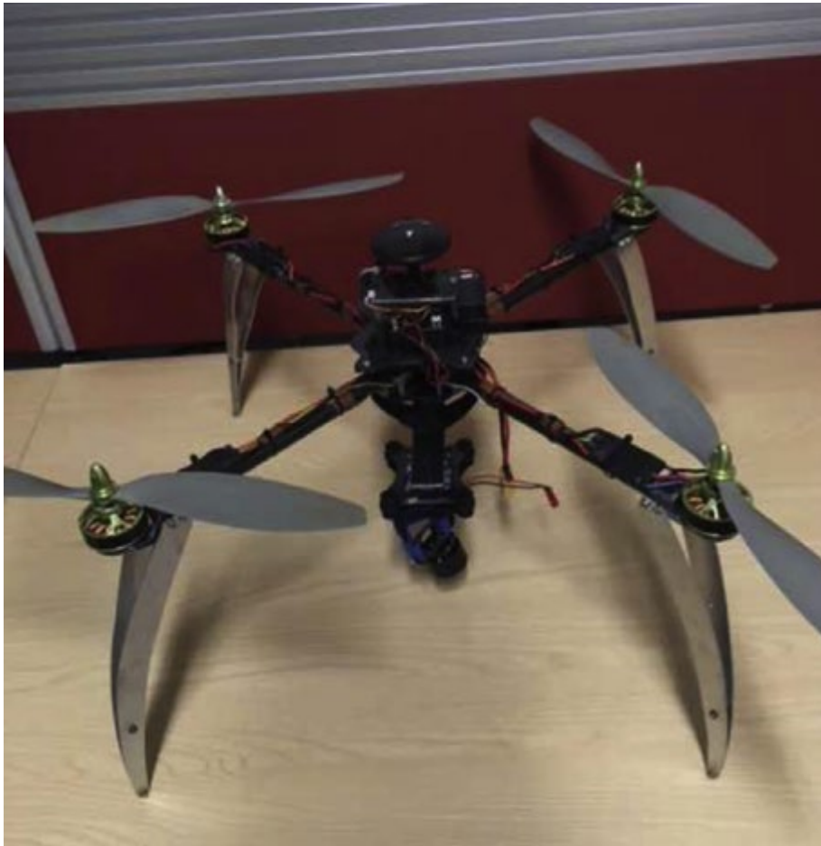
Figure 6: Quadcopter UAV with attached radiation monitoring package as used in Fukushima related monitoring activities (reproduced from Connor et al., 2018).
