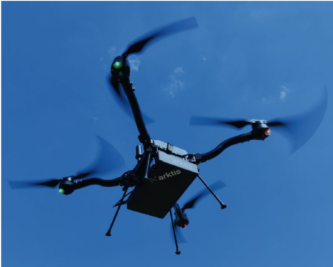
Figure 5: Commercially available multi-rotor UAV with radiation monitoring payload from Arktis (reproduced from Arktis, 2025).
