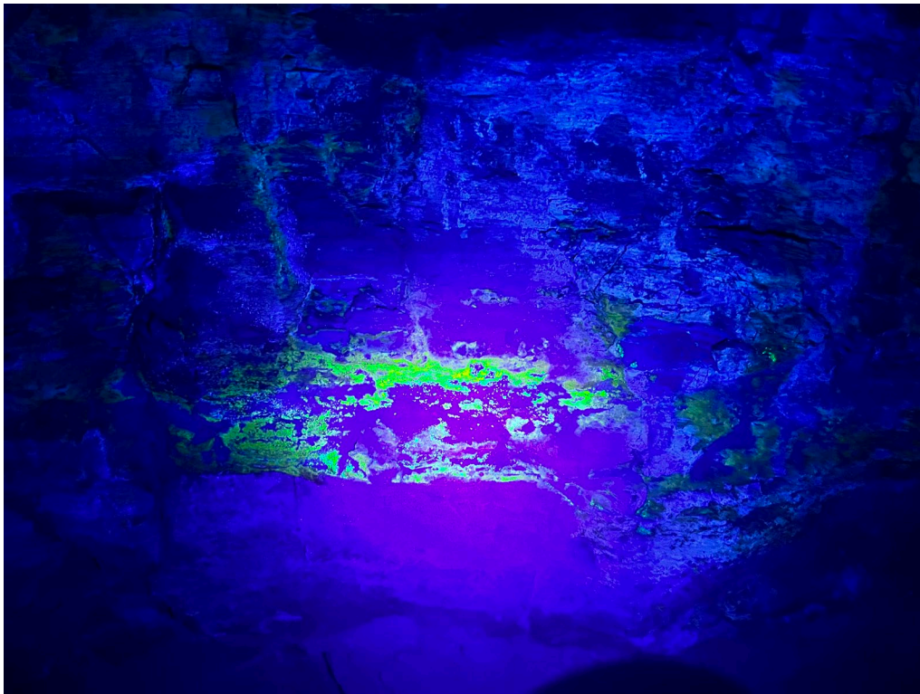
Figure 24: UV map of fluorescent uranyl mineral precipitates inside the former Sue mine in Arizona (reproduced from Verbelen, 2024).
