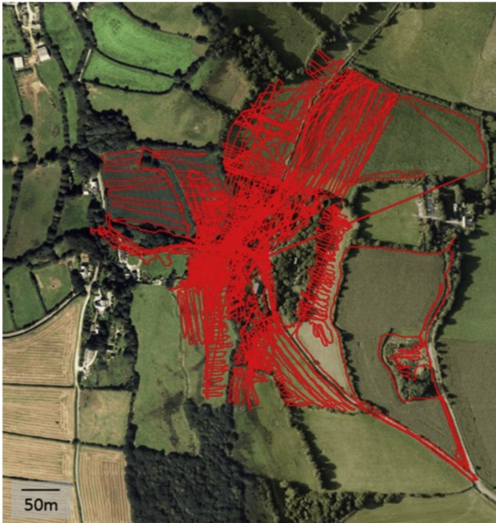
Figure 15: Satellite image overlain with the flight path of a UAV during a survey of the former South Terras mine in Southwest England (reproduced from Martin et al., 2015).
