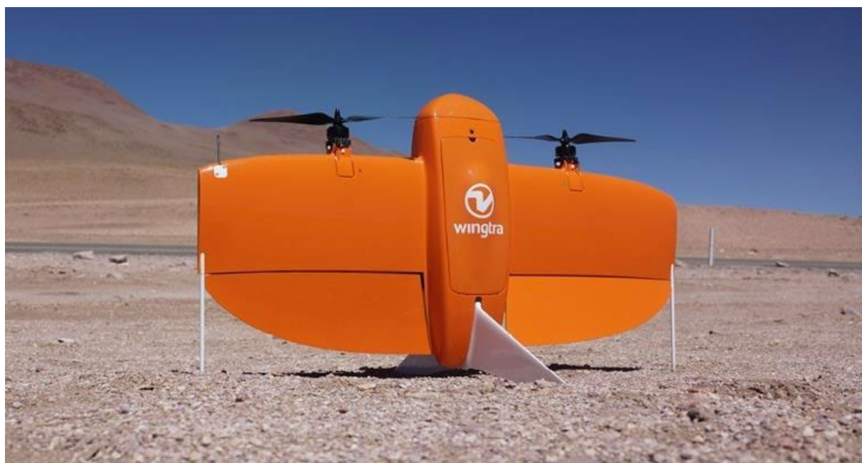
Figure 1: Wingtra vertical take-off and landing (VTOL) fixed-wing UAV (reproduced from Woodbridge et al., 2023).
