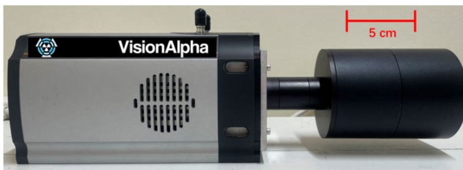
Figure 25: Long-range alpha detection camera patented by VisionAlpha (reproduced from VisionAlpha, 2025a).
