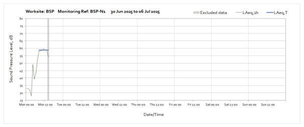
Note: Missing data from 15:00 on Monday  $30^{th}$  June until the end of the month was due to a failed restart of the monitoring station.
