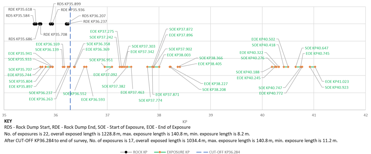
Figure 3.4.5: PL1965 & PL1966 rock vs. exposure detail (2017) 7
