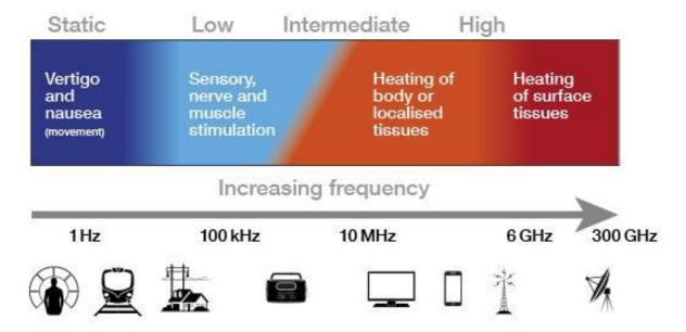
Exposure to high levels of EMF can give rise to effects that may be irritating of unpleasant. The effects in a particular case depend on the frequency range and intensity of the EMFs to which a worker is exposed.
