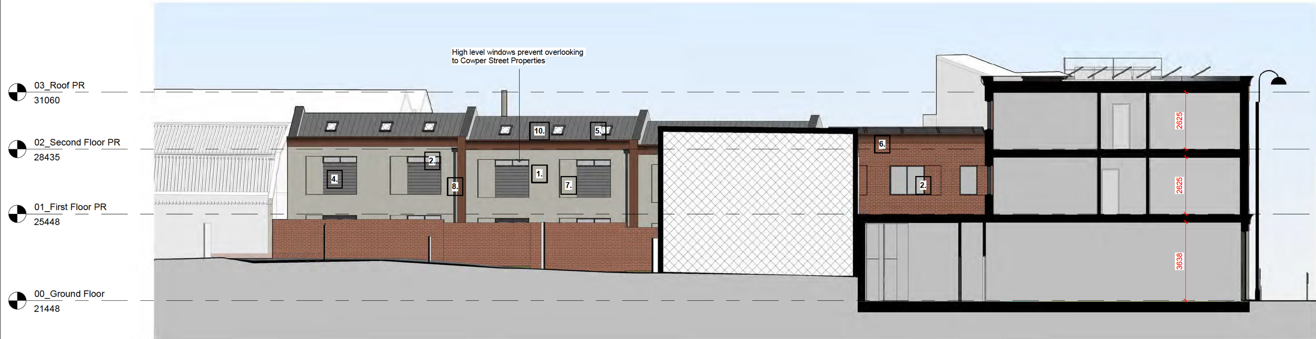
East Sectional Elevation - Proposed (SE1)
