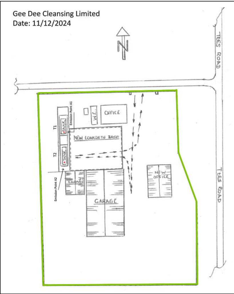
Figure 2: Site Layout Plan including emission points
