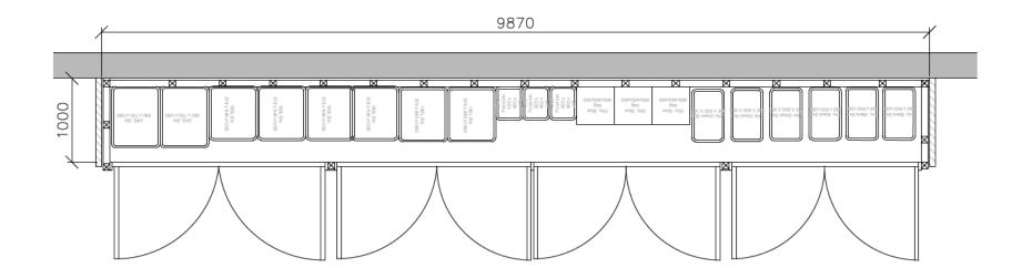
Timber boarded and felt roof bin store. Louvered timber doors to bin areas with hinged roof portions for easy refuse deposit.
