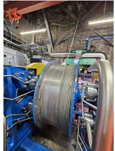
Above Installation of new winding engine that operates the cage that goes underground in the mine experience.
