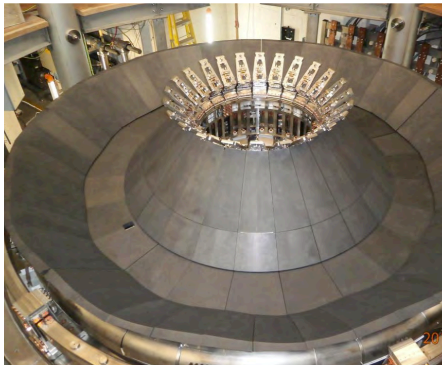
The lower divertor cryopump on MAST Upgrade as the device was under construction.
