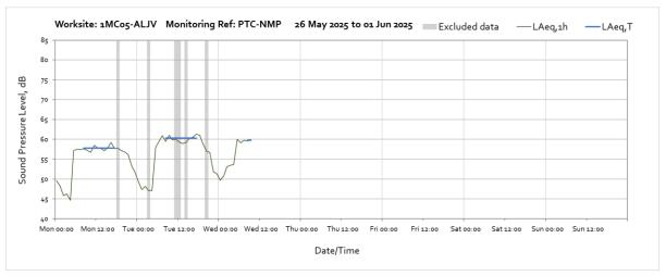
Note: Missing data between 10:00 on Wednesday 28<sup>th</sup> May and the end of the month was due to the a fault with the timing system following replacement of monitoring station.
