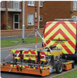
Large-scale ground-penetrating radar can be attached to a van. Image courtesy of Macleod Simmonds.
