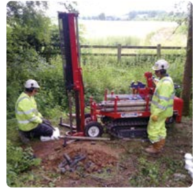
A motor-driven hammer pushes a cone into the ground for dynamic probing. Image courtesy of CH2M.
