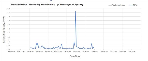
Note: Missing data between 12:00 on Friday  $4^{th}$  April and 12:00 on Tuesday  $8^{th}$  April was due power loss at the monitoring station caused by local power failure.
