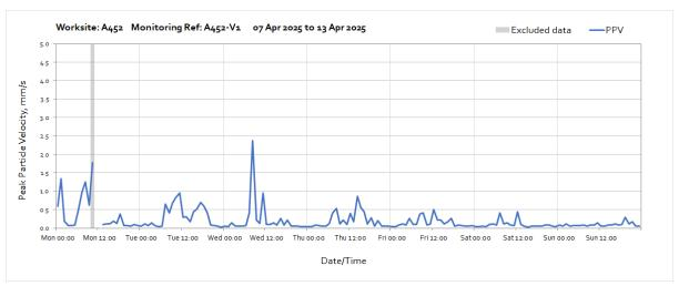
Note: Missing data between 11:00 and 13:00 on Monday 7<sup>th</sup> April was due to field calibration of the monitoring station.
