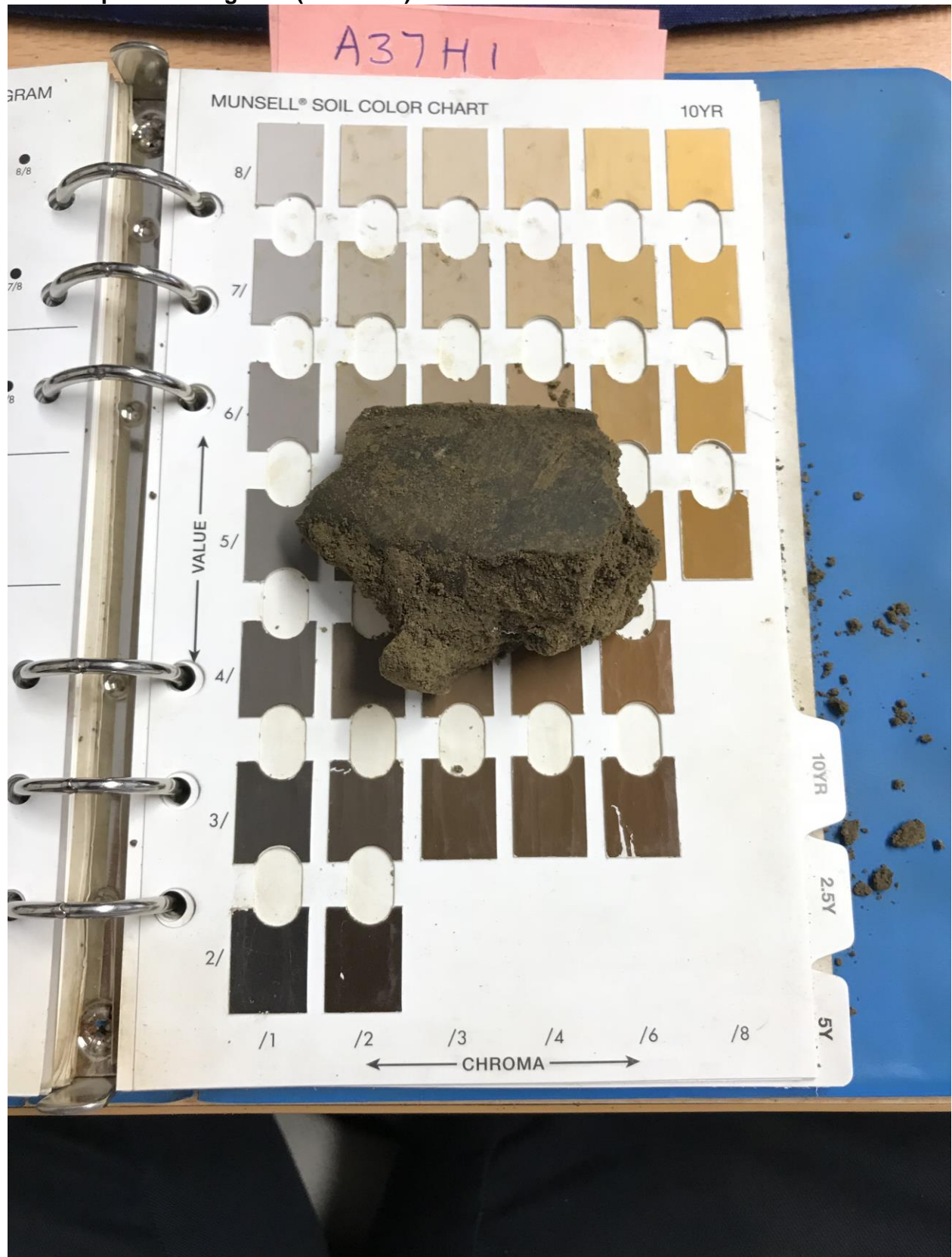
Soil Sample from Auger 37 (Horizon 1) with Munsell Chart
