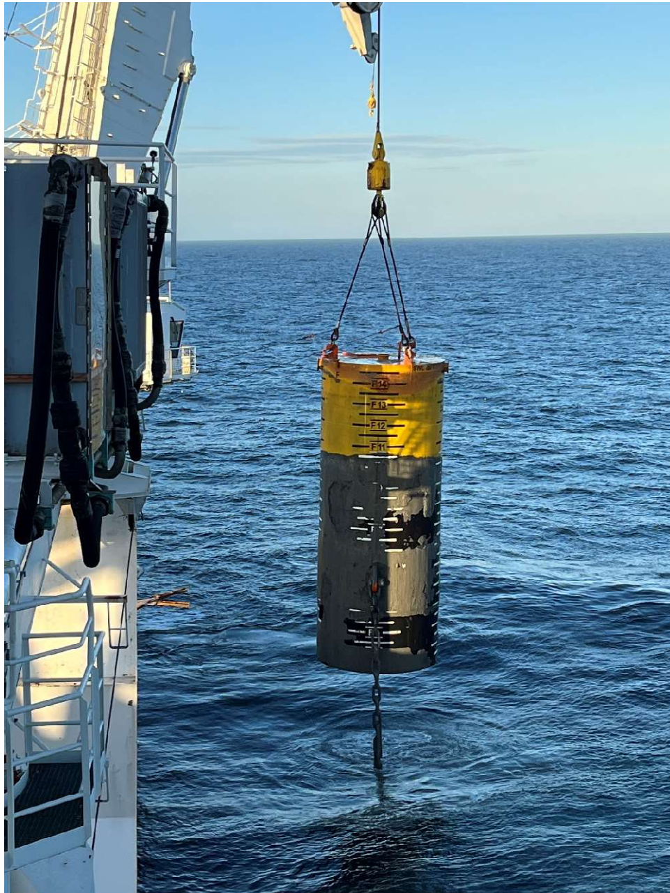
Figure 8.1.2: Suction anchor recovery to vessel
