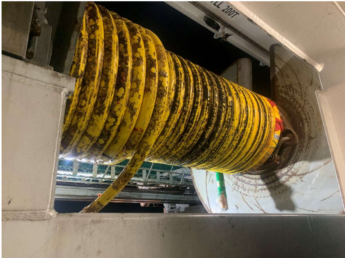
Figure 8.8.3: Riser recovery, drum
