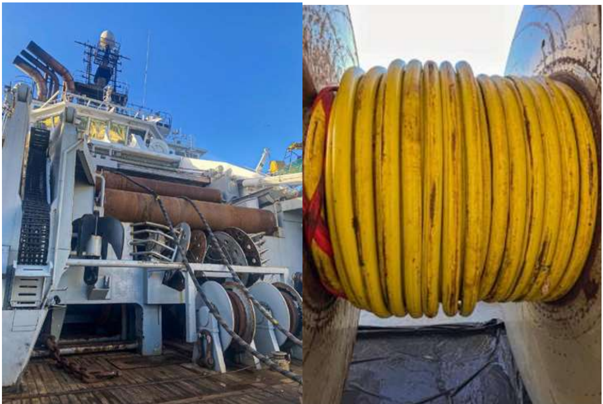
Figure 8.7.3: Product spooling (left) & storage on drum (right)
