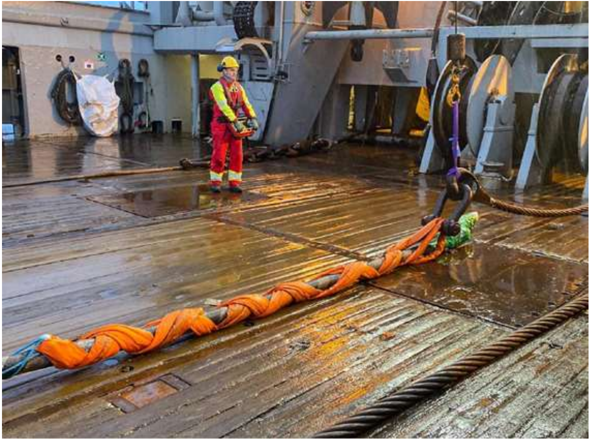
Figure 8.7.2: Chinese finger used to recover flexible risers
