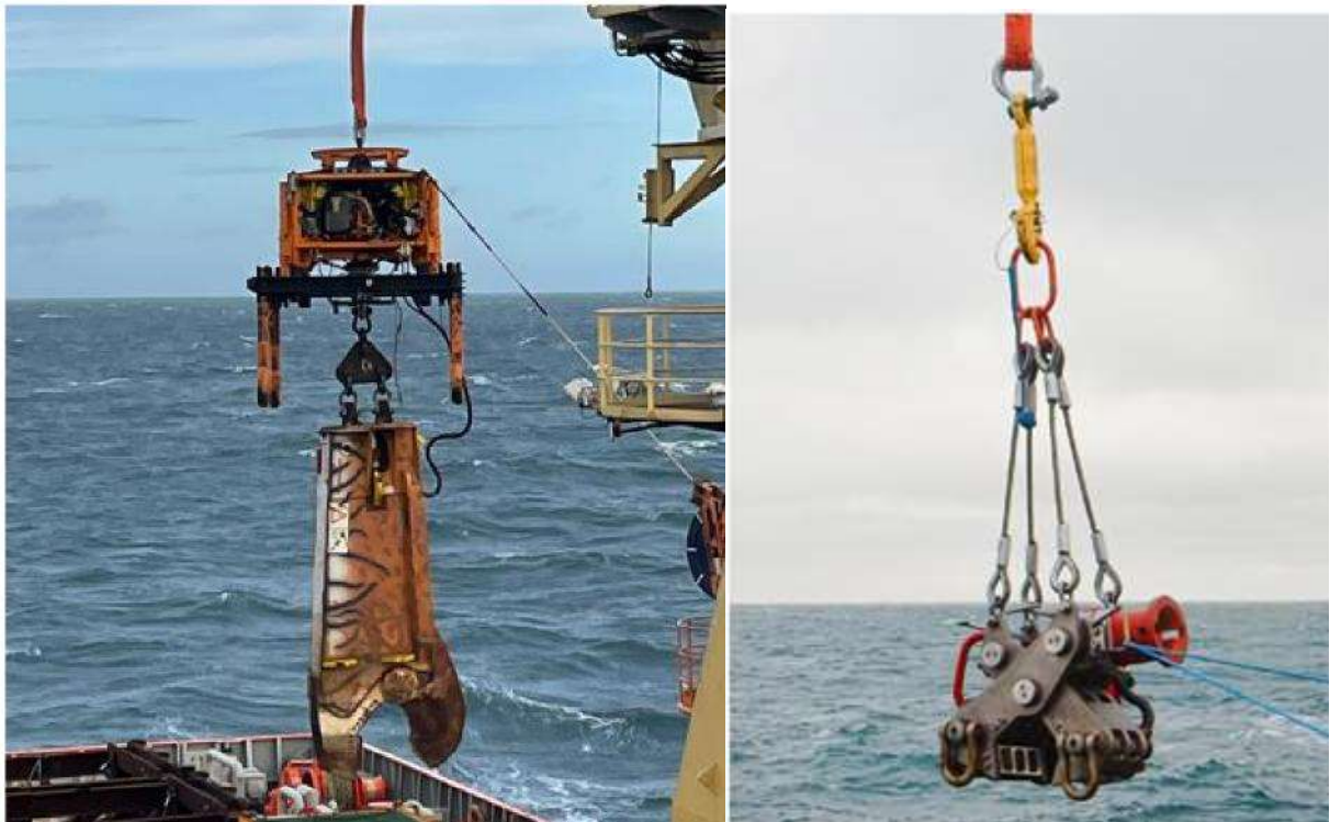
Figure 8.7.1: UTROV™ & shear cutter (left), CRT200 pipe clamp (right)
