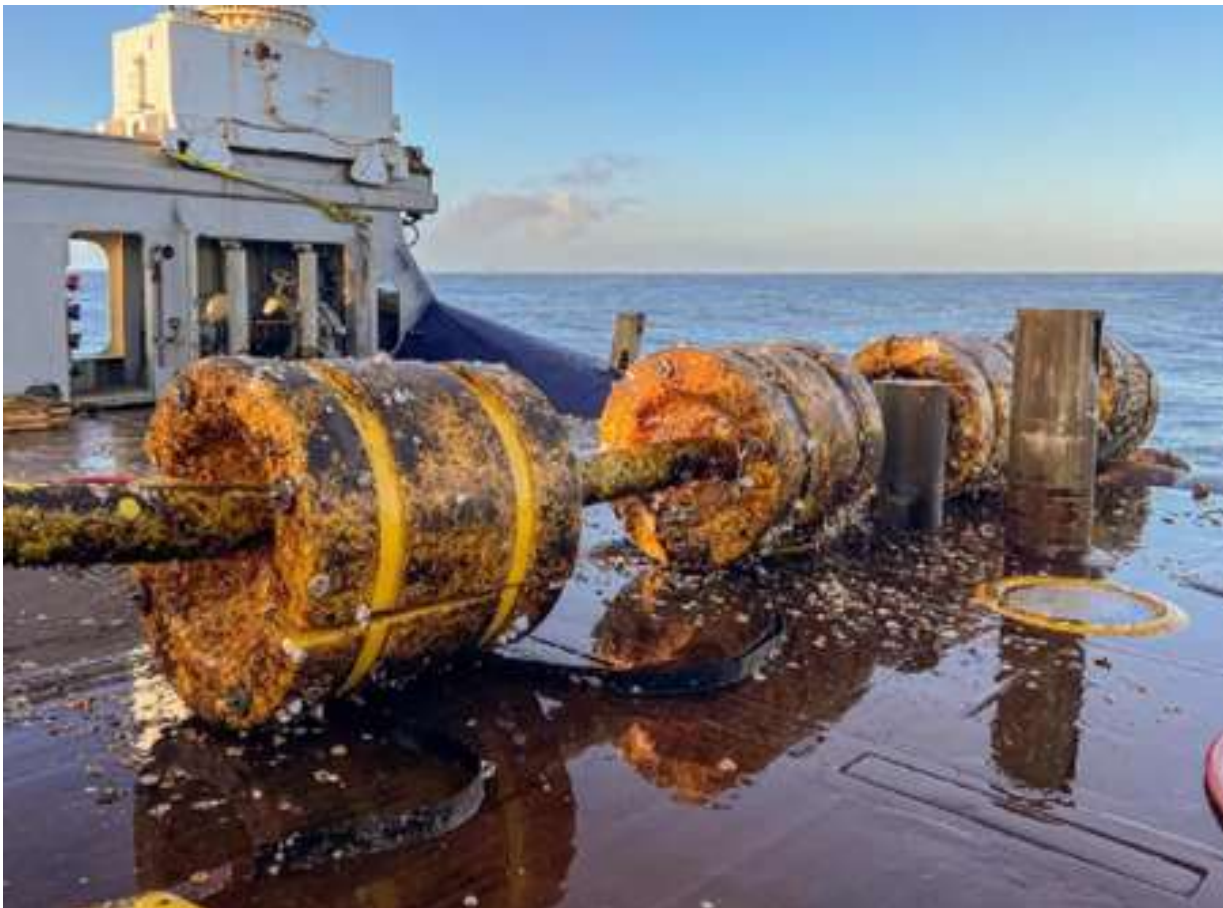
Figure 8.8.1: Buoyancy modules on deck following recovery
